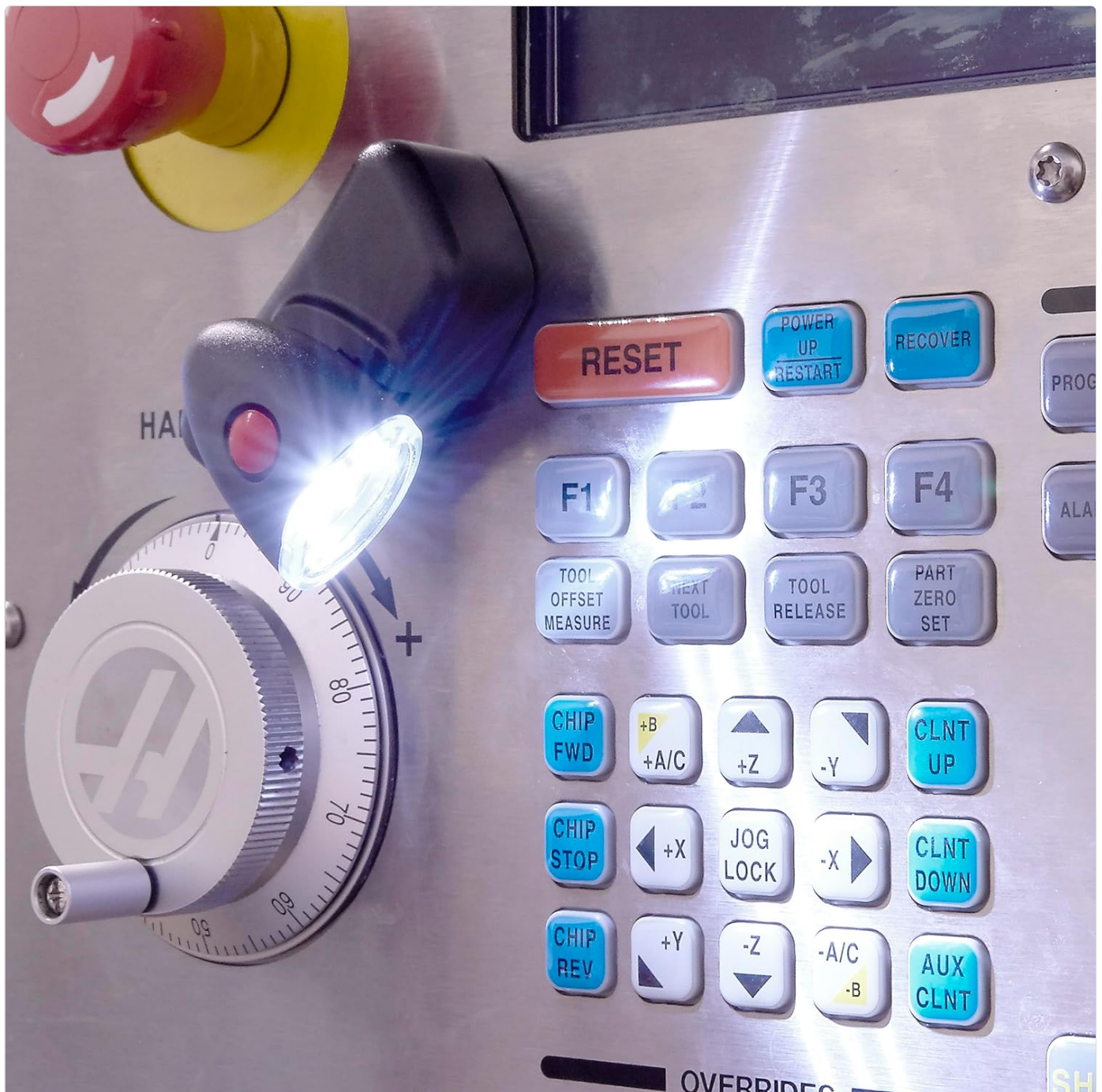
Image 4.2: The LED lamp detached from the visor, demonstrating its use as a portable, free-standing light source with its magnetic base.
