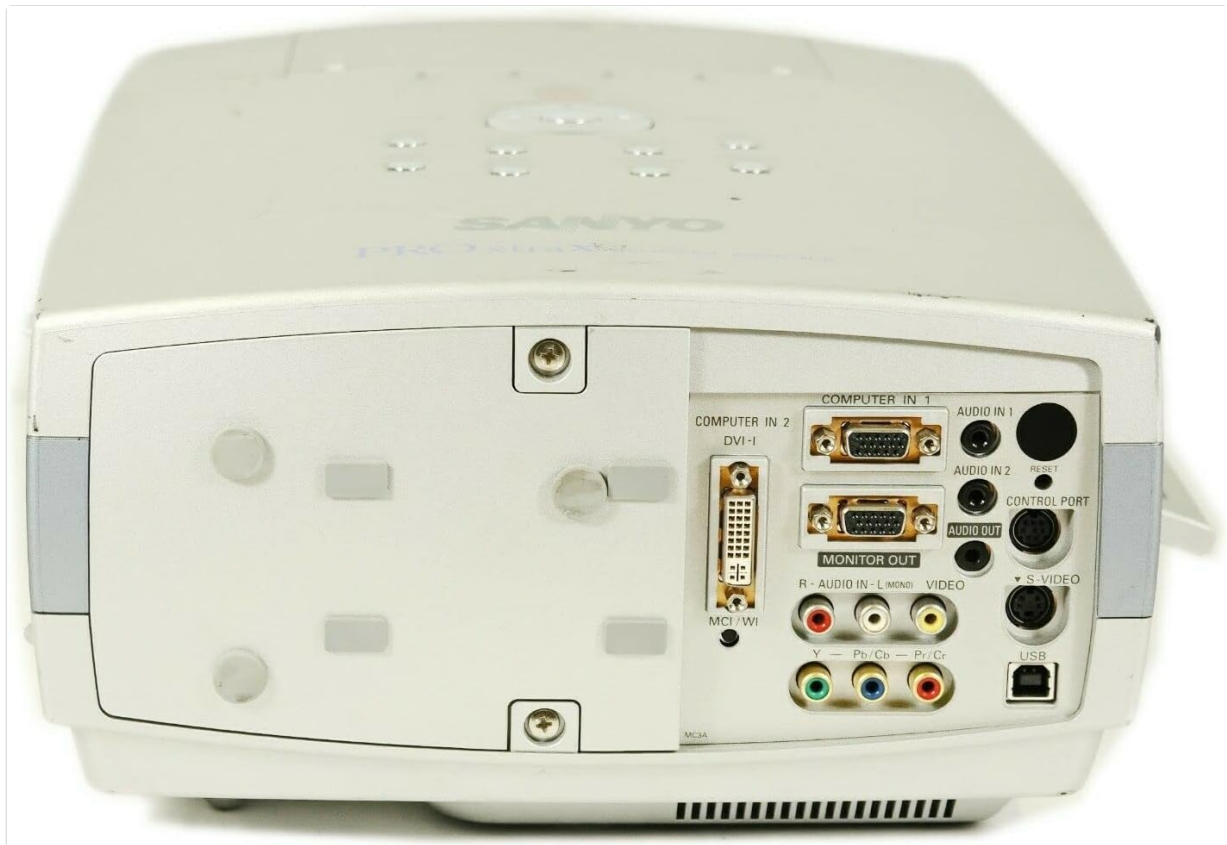
Figure 4.2: Rear Connection Panel. This image provides a clear view of the projector's rear panel, detailing the various input and output ports including Computer In (VGA), DVI-I, Audio In/Out, Monitor Out, S-Video, Video, and USB ports.
