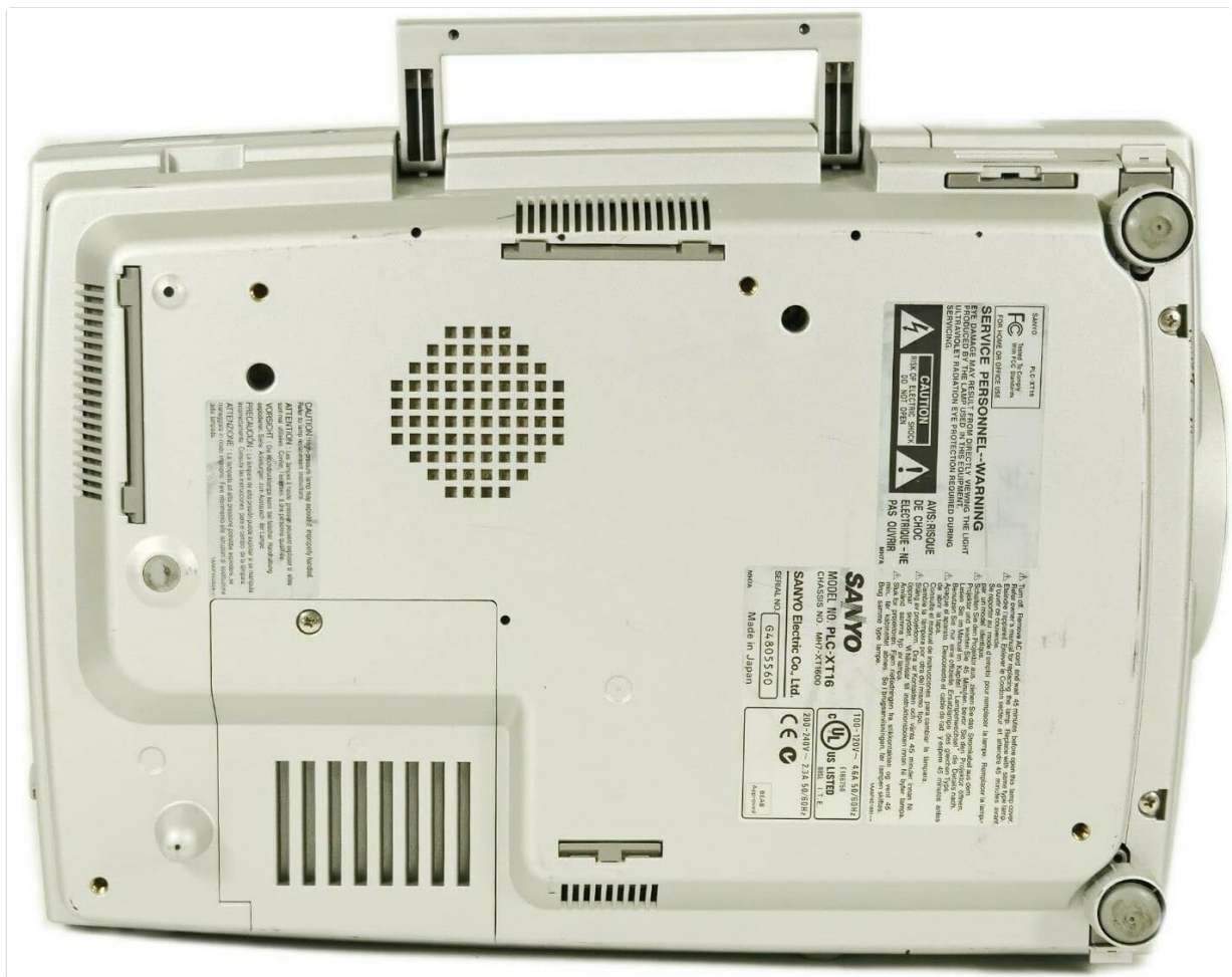
Figure 4.5: Bottom View. This image shows the underside of the Sanyo PLC-XT16 projector, including the adjustable feet for leveling and the product information label detailing model number and electrical ratings.
