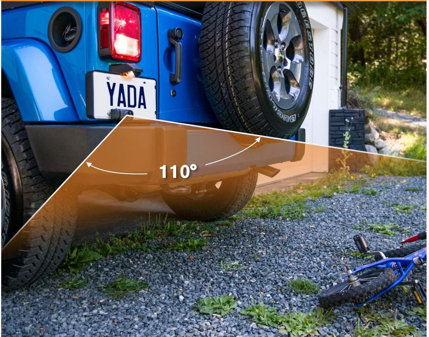
Image: An illustration demonstrating the 110-degree wide-angle view provided by the YADA backup camera, showing a broad perspective behind the vehicle.
