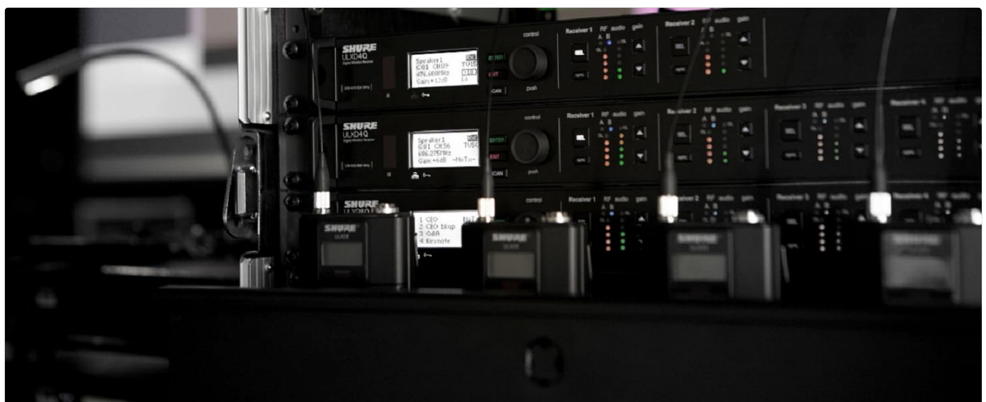
Image: A rack-mounted Shure ULXD4 receiver unit alongside ULXD1 bodypack transmitters and handheld microphones, illustrating a complete wireless system setup.
