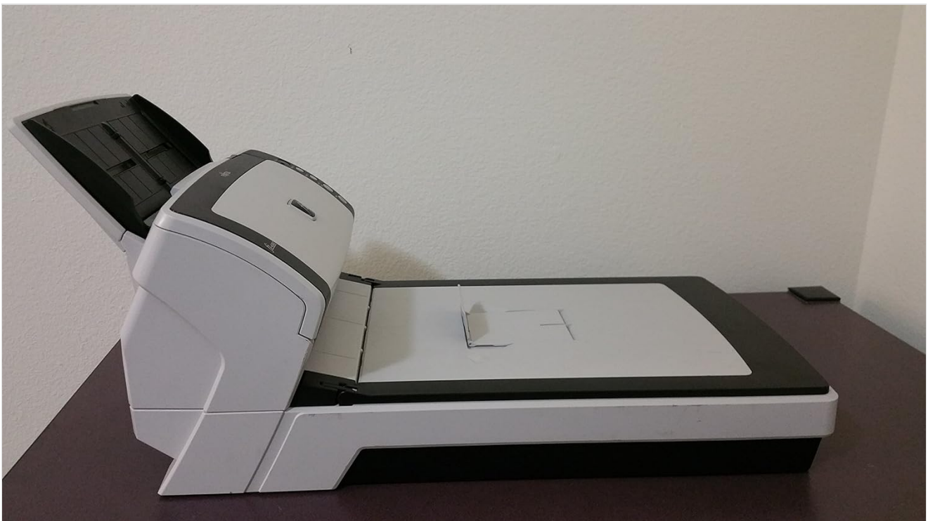
Figure 3: Side view of the scanner with the ADF input tray extended, ready for document loading.
