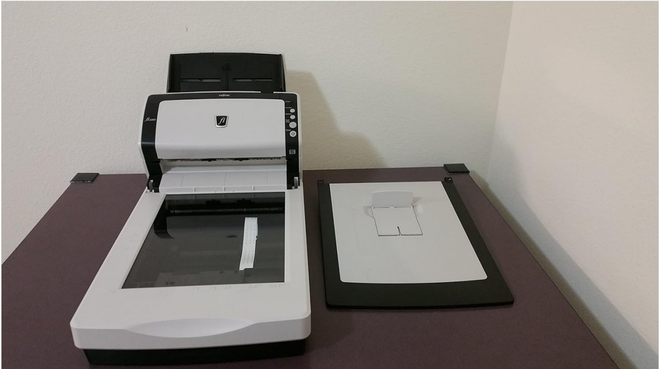
Figure 5: The flatbed unit detached from the ADF unit, illustrating its modular design.
