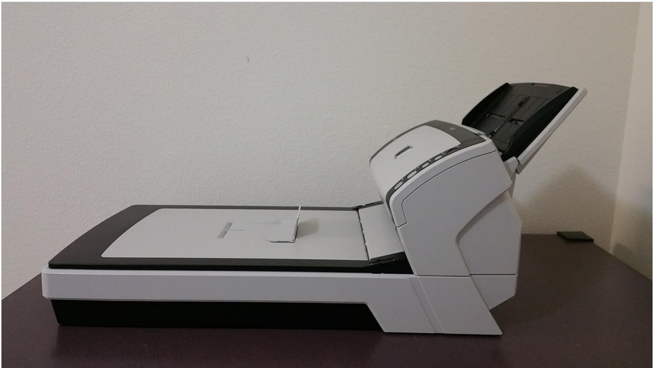
Figure 1: Side view of the Fujitsu Fi-6240Z scanner, showing the flatbed on the left and the Automatic Document Feeder (ADF) on the right.
