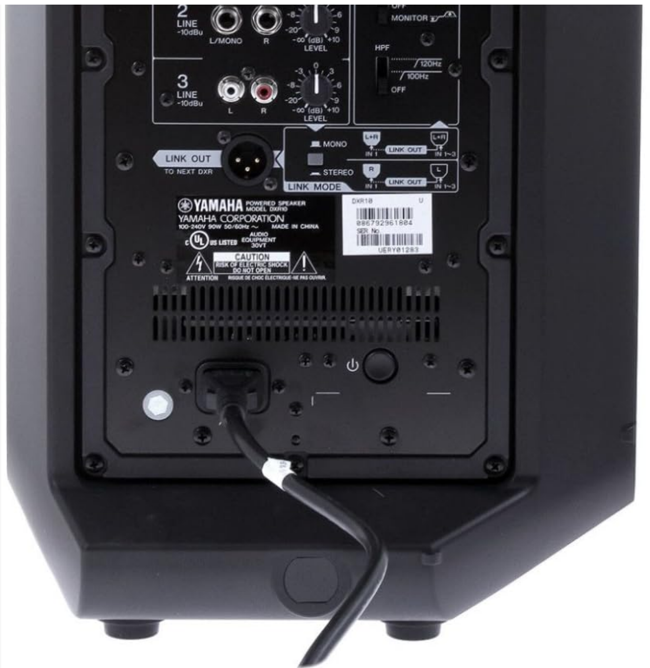
Figure 3: Rear panel of the DXR 10, illustrating the power input and control section.
