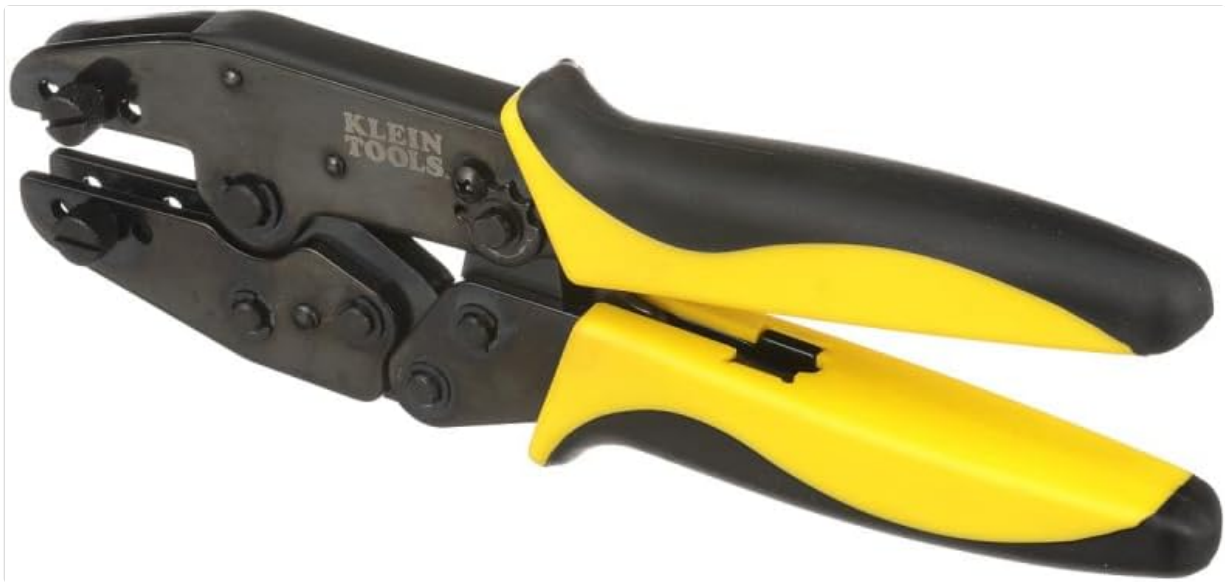
Figure 3: Angled view of the Klein Tools VDV200-010 Ratcheting Crimper Frame, illustrating the area where interchangeable die sets are installed and secured with thumb-screws.
