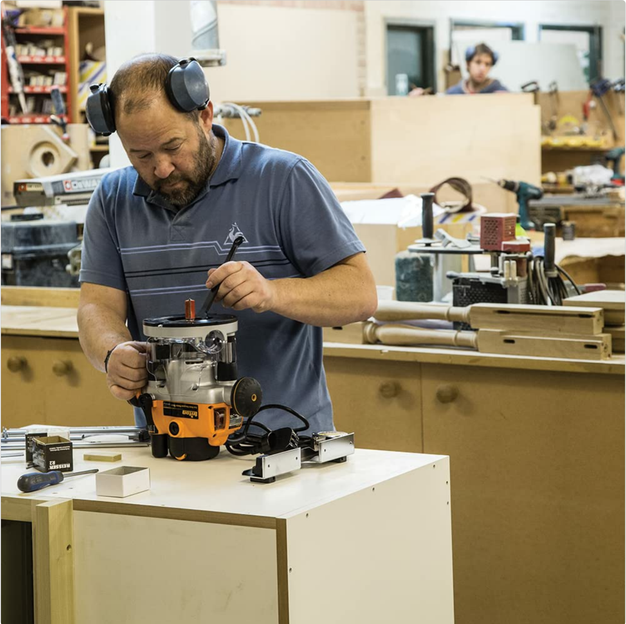
Image: A user installing a router bit into the Triton MOF001, highlighting the ease of bit change.
