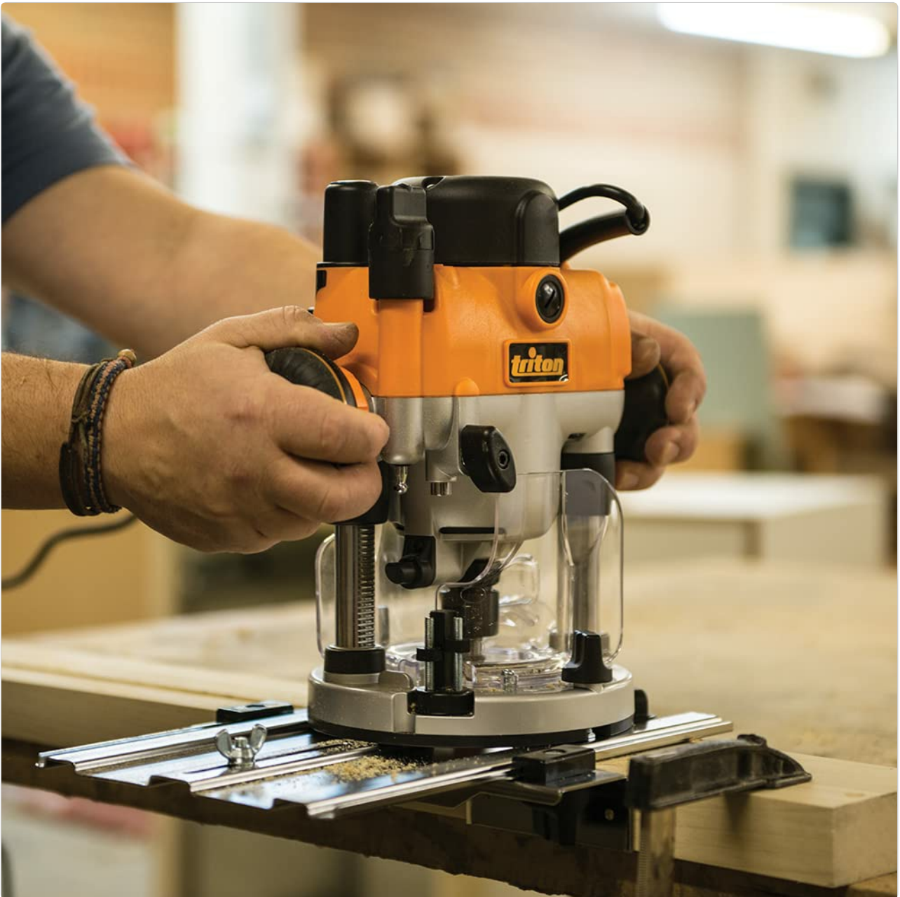
Image: A user performing a handheld routing operation with the Triton MOF001 and a guide fence.
