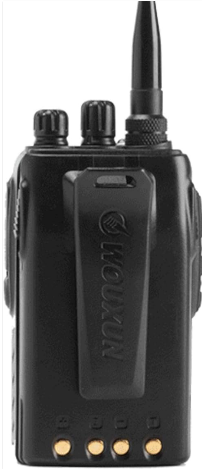
Image: Rear view of the Wouxun KG-UV6D radio, showing the attached belt clip and the battery compartment. The gold contacts for charging are also visible at the bottom.
