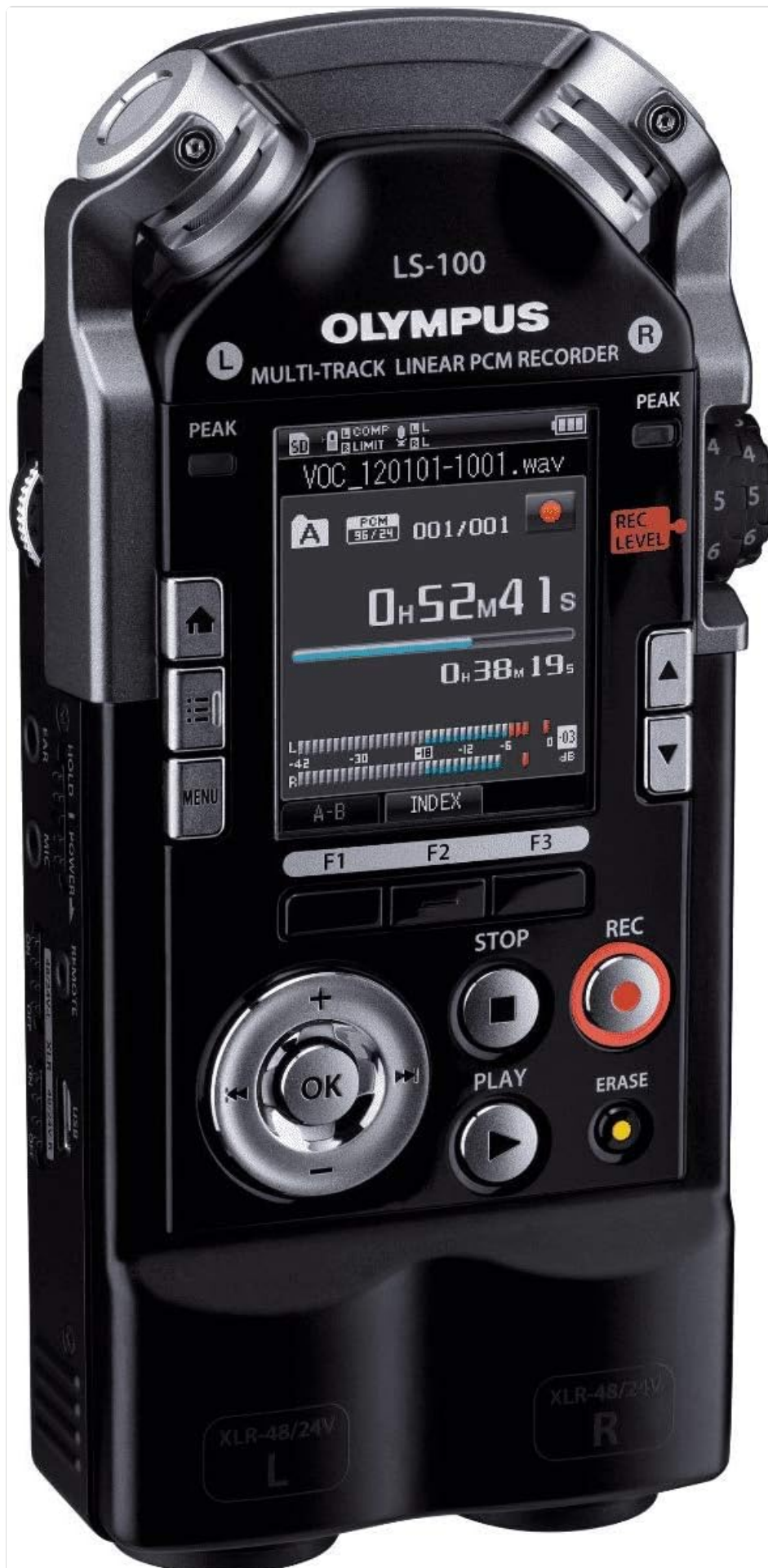
Image: Front view of the Olympus LS-100 Voice Recorder, showing the display, control buttons, and built-in microphones.
