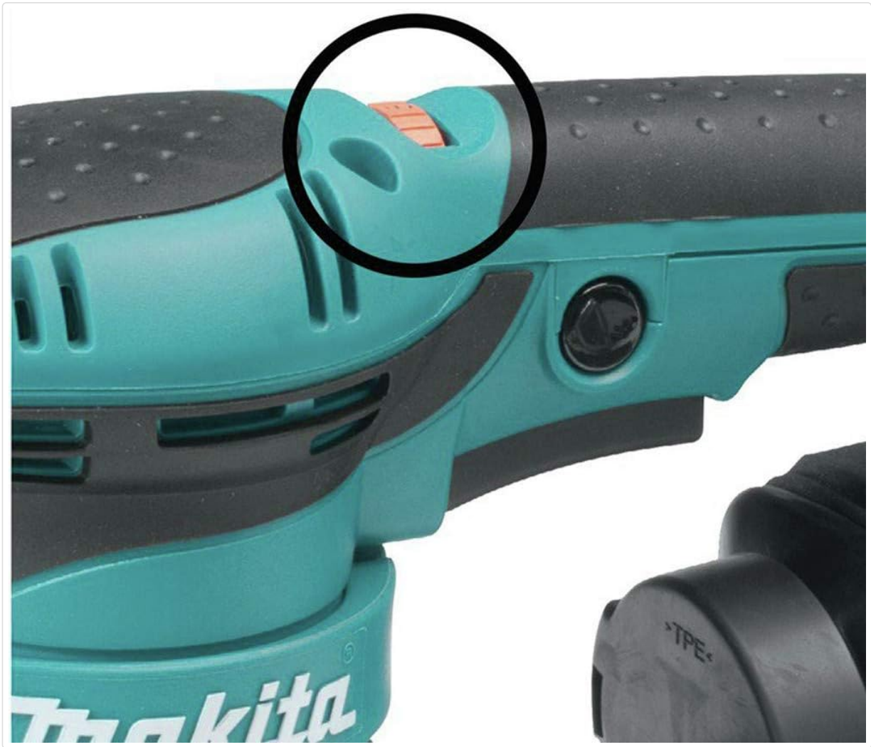
Figure 3: The variable speed control dial, allowing adjustment of sanding speed from 4,000 to 12,000 OPM.
