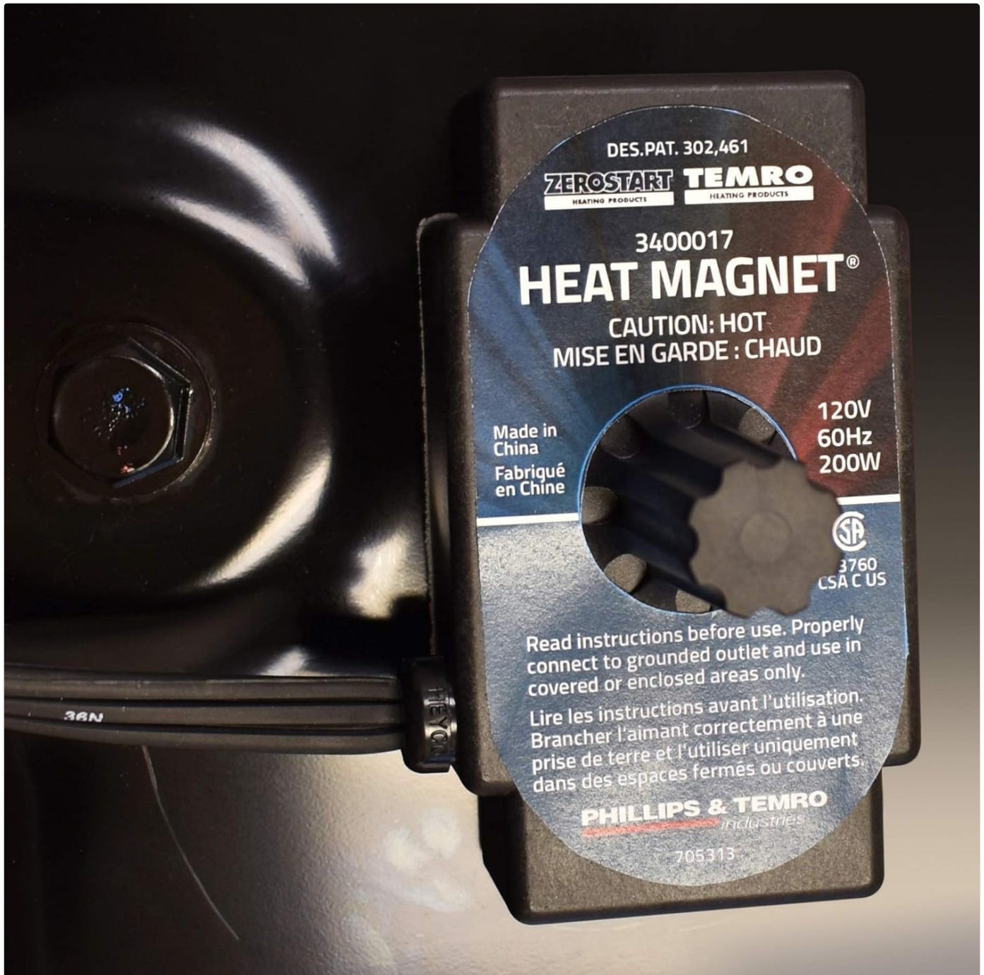
Figure 2: Close-up of the product label, indicating 120V, 60Hz, 200W power specifications and CSA certification. This label also includes a caution for hot surfaces.
