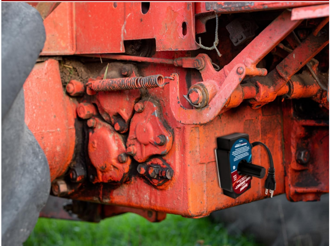
Figure 4: The ZeroStart Heat Magnet Heater attached to a metallic surface on a tractor, demonstrating its application for pre-heating engine components.
