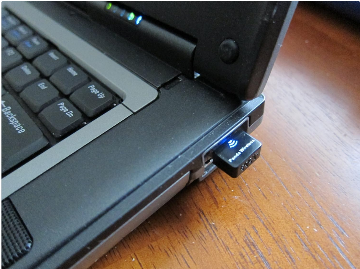
Image 2.2: The Panda Wireless USB Adapter installed in a laptop's USB port, showing its compact design.
