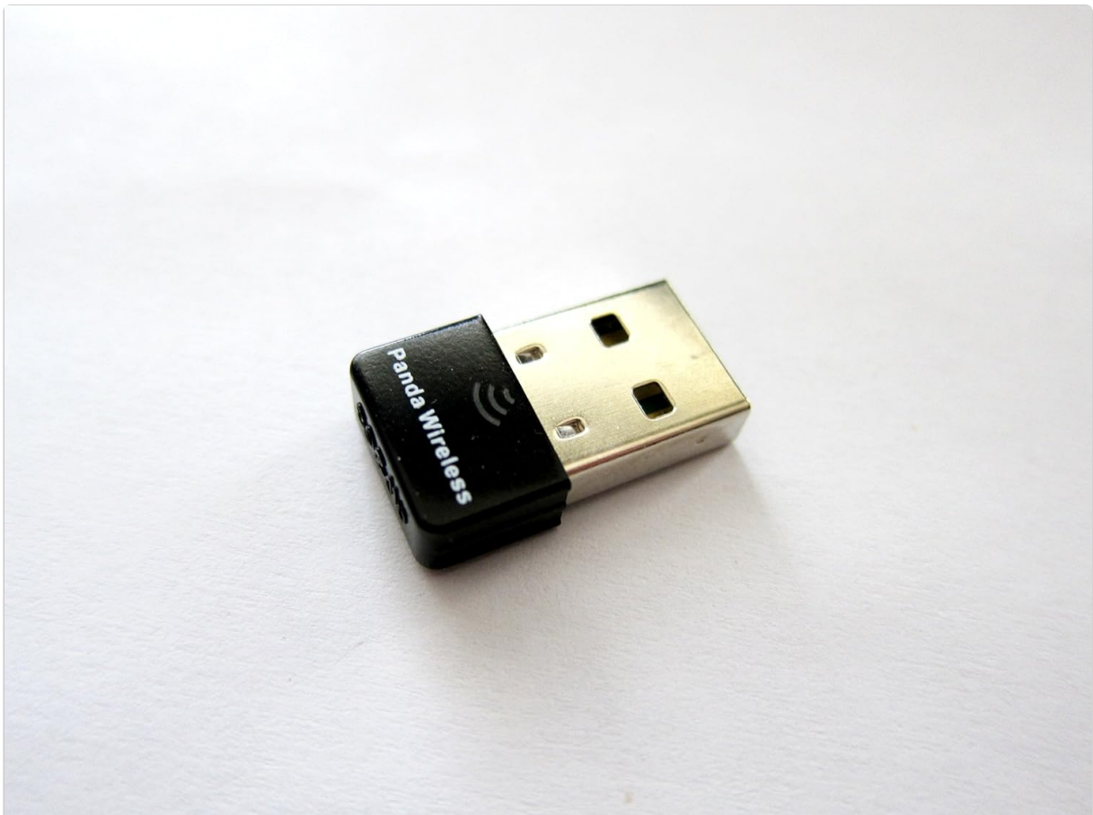
Image 1.1: The Panda Wireless Ultra WiFi 150Mbps Wireless-N 2.4GHz USB Adapter (Model PAU03).
