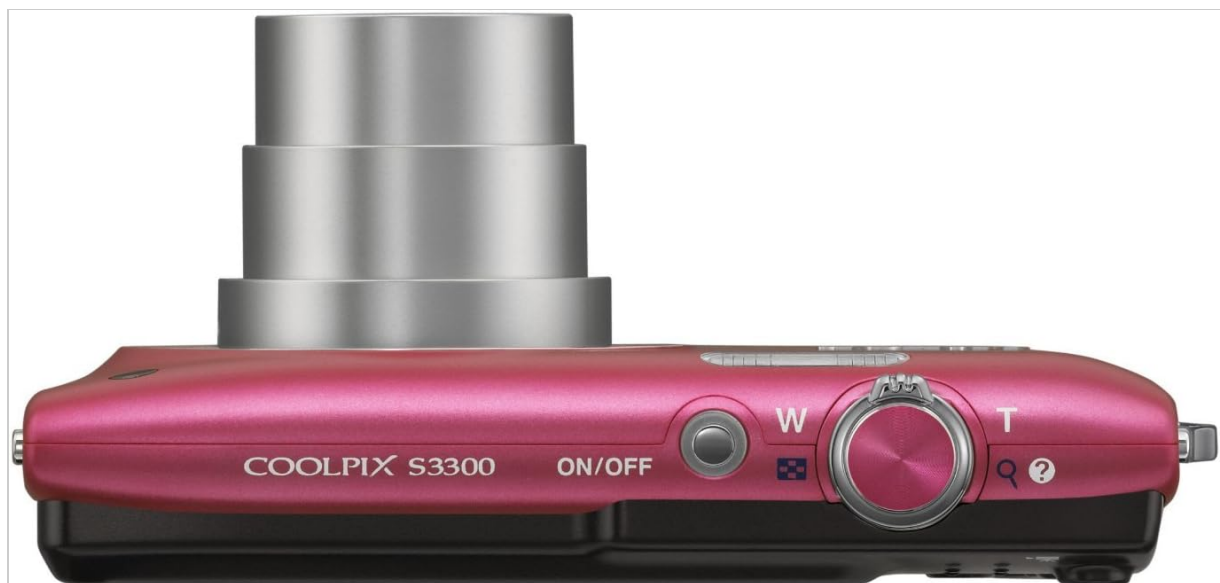
Image 2: Top View of Nikon COOLPIX S3300. This image shows the top of the camera, featuring the power button, shutter button, and zoom lever (W/T).
