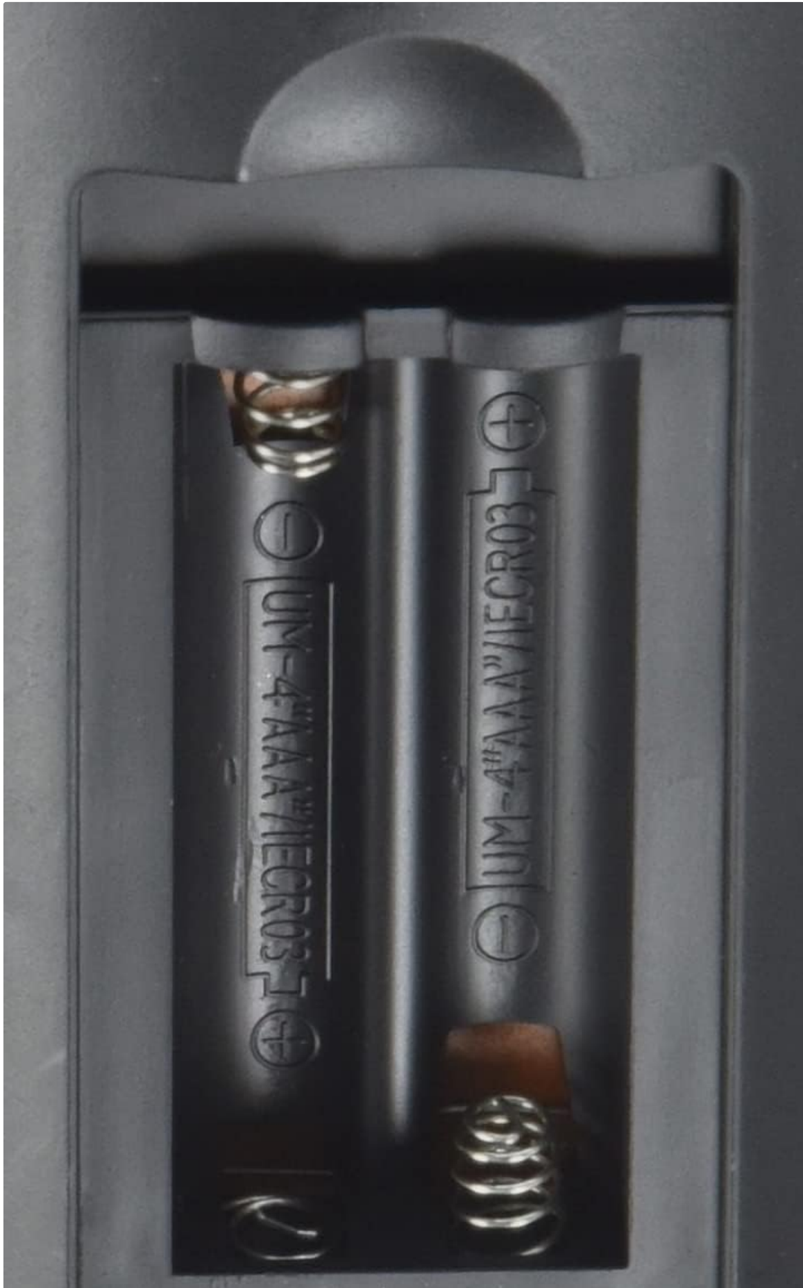
Image: Close-up view of the battery compartment, clearly indicating the requirement for AAA batteries and their correct orientation.
