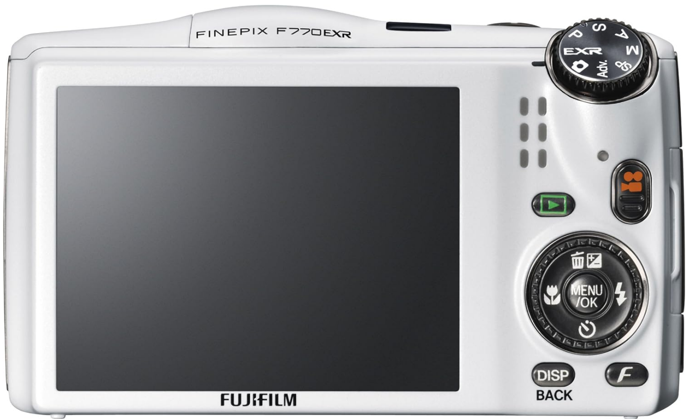
Figure 2.3: Back View. This image presents the rear of the camera, featuring the large LCD screen, navigation buttons, menu button, and mode dial, which are essential for camera operation and settings adjustment.
