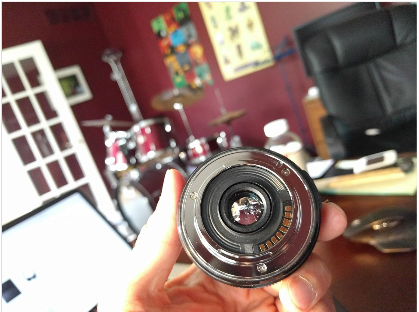
Figure 3: Rear View. This image presents the rear of the Samsung NX 16mm f/2.4 lens, detailing the lens mount and electronic contact pins for communication with the camera body.
