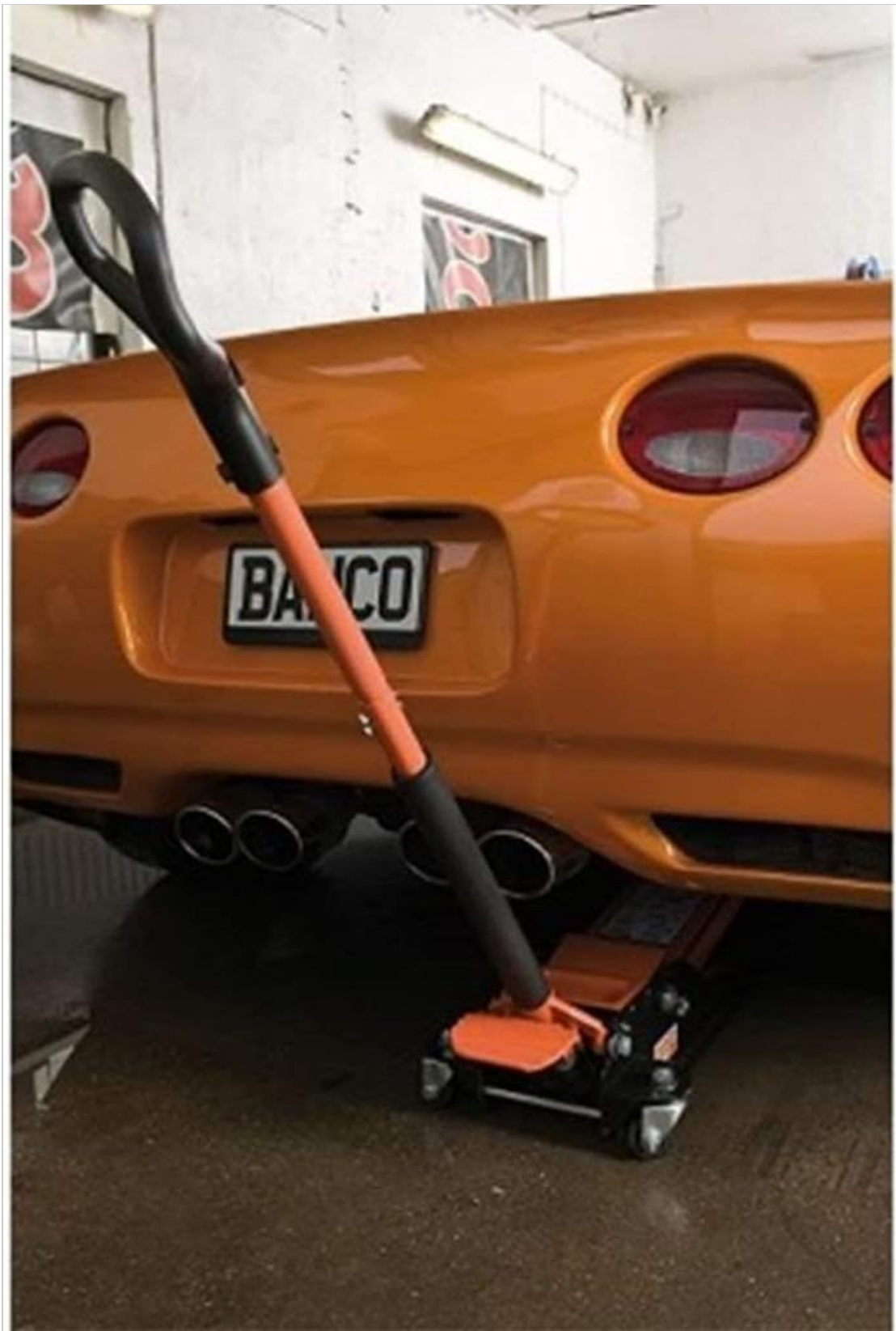
Figure 3: Bahco BH12000 Jack positioned under the rear of a vehicle. This image demonstrates the jack's low profile and its application for lifting a car.
