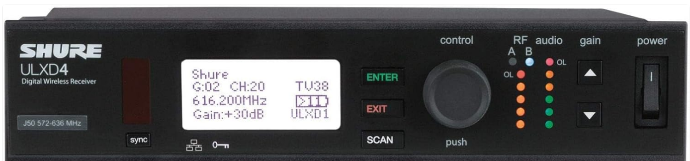
Figure 1: Front panel of the Shure ULXD4 Single Channel Receiver, showing the display, control knob, and various indicators.
