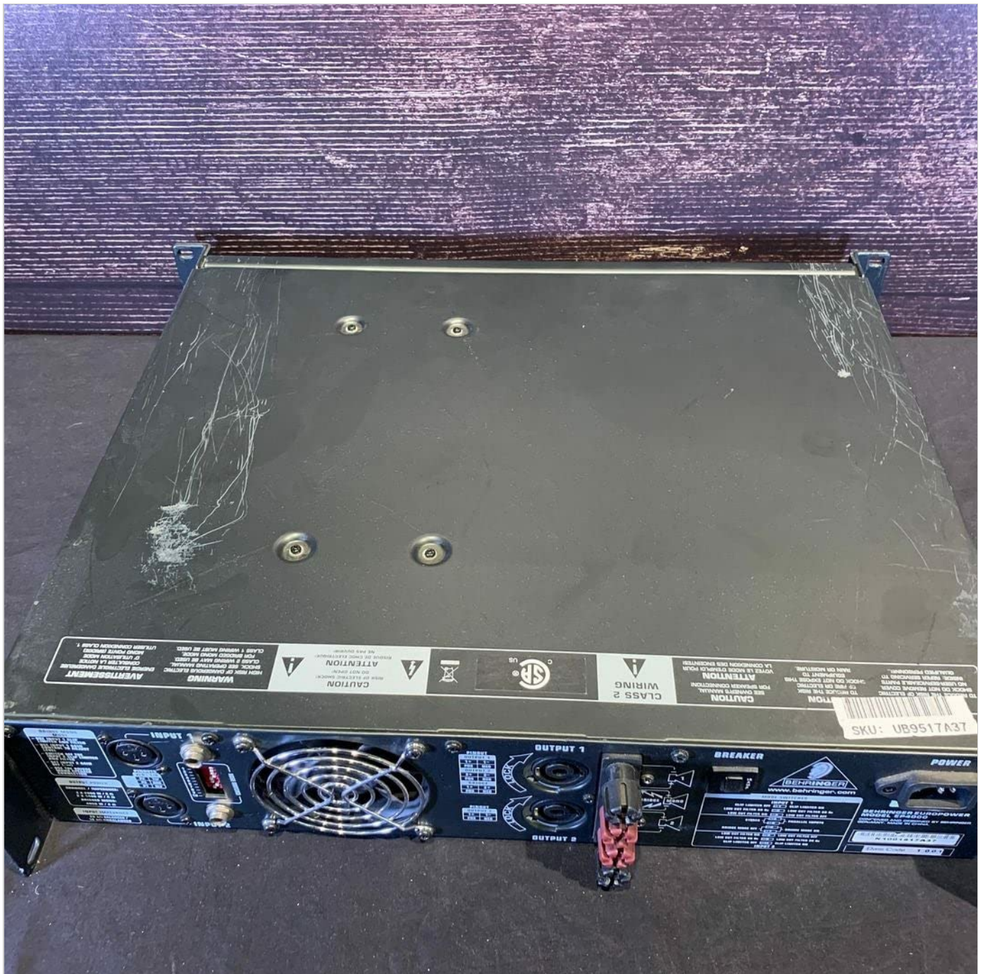
Figure 2: Rear panel of the Behringer EP4000 Power Amplifier. This view displays the input connectors (XLR and 1/4" TRS), output connectors (Speakon and binding posts), mode switches (stereo, parallel, bridge), and the power input with a circuit breaker.
