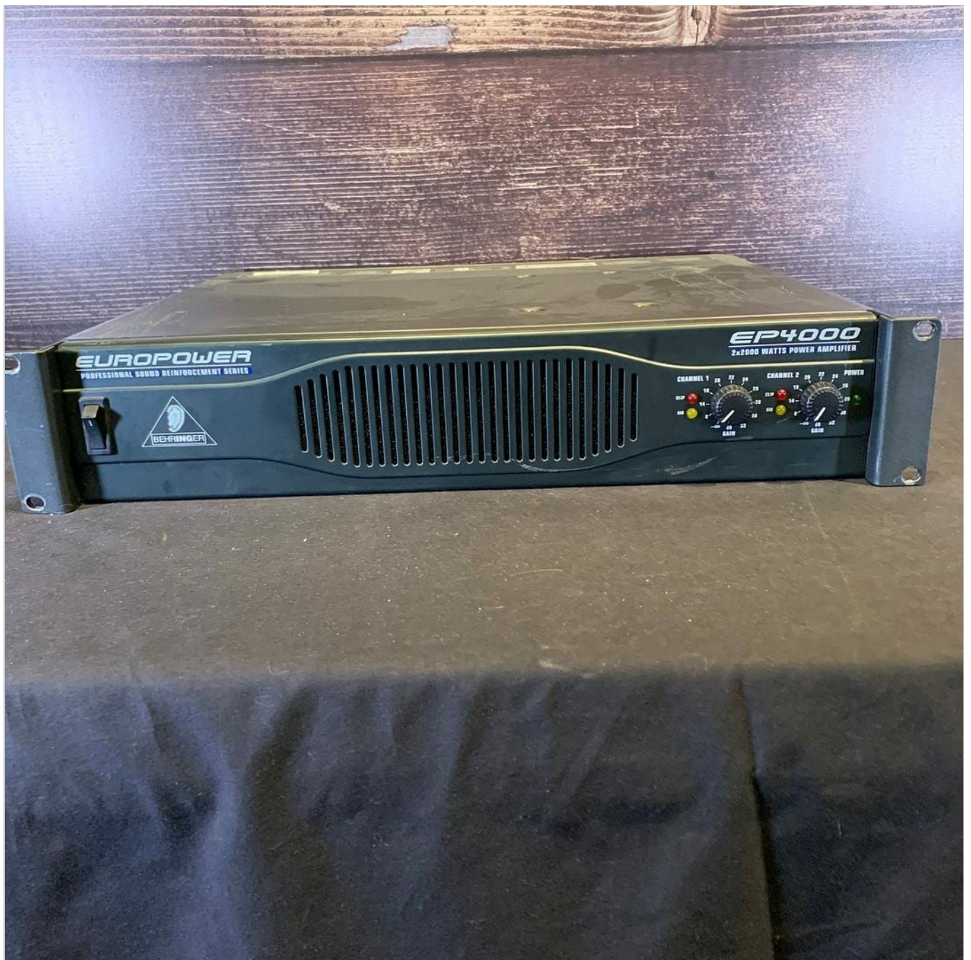
Figure 1: Front panel of the Behringer EP4000 Power Amplifier. This view shows the power switch, ventilation grille, and control knobs for Channel 1 and Channel 2, including gain controls and LED indicators for signal, clip, and protection.
