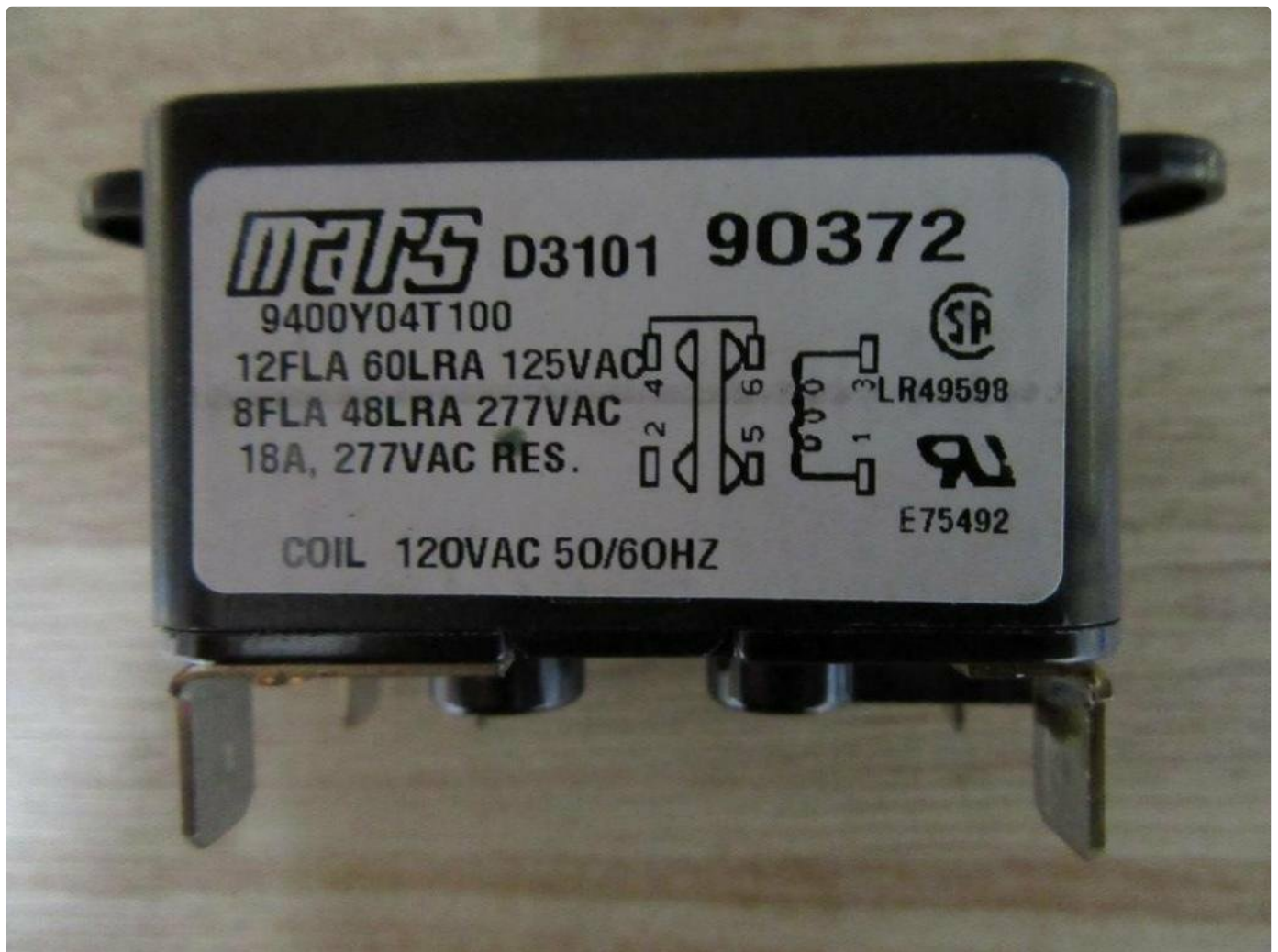
A detailed view of the MARS 90372 relay's top label. The label specifies the model D3101 90372, along with electrical ratings: 12 FLA, 60 LRA at 125 VAC; 8 FLA, 48 LRA at 277 VAC; and 18A, 277 VAC resistive. It also indicates a coil voltage of 120 VAC 50/60HZ and includes UL and CSA certifications.
