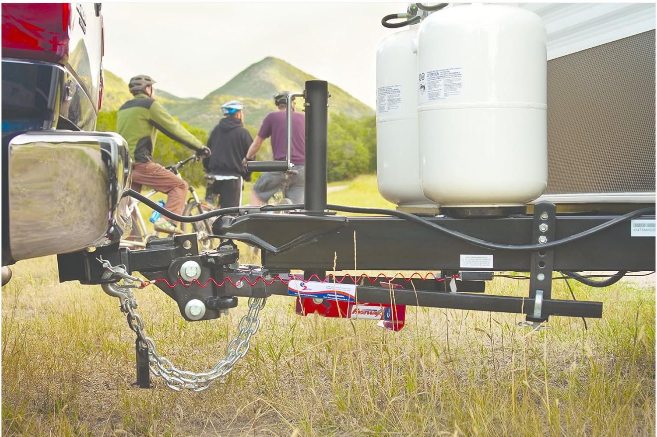
Figure 5: A trailer hitched to a tow vehicle with the Fastway Zip breakaway cable properly installed, ready for towing.
