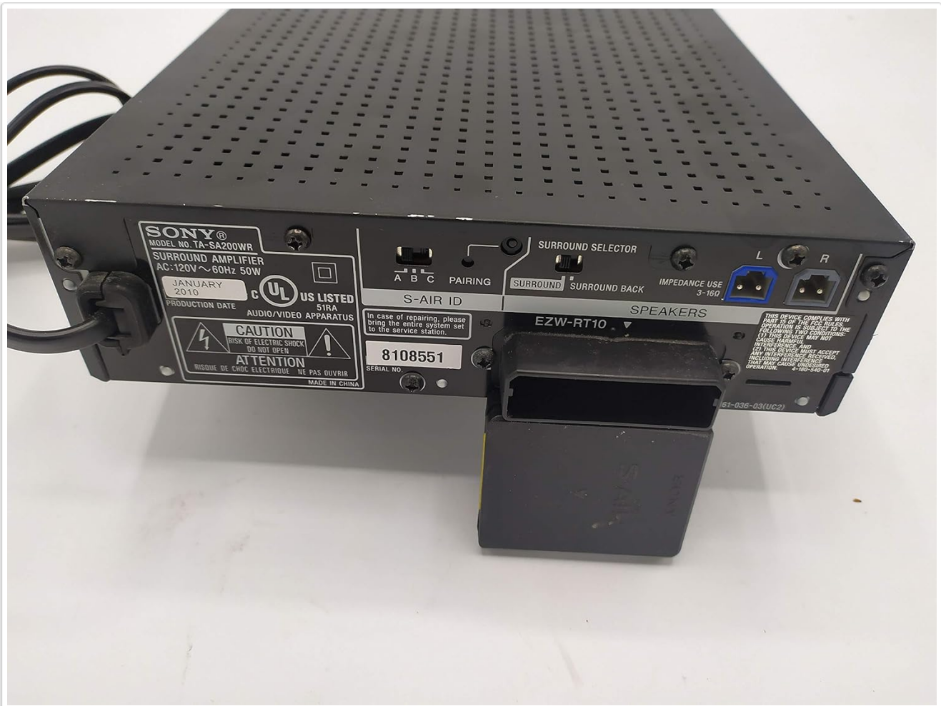
Figure 2.2: Rear panel of the TA-SA200WR, highlighting the speaker output terminals (L/R) and the S-Air ID selector switch.
