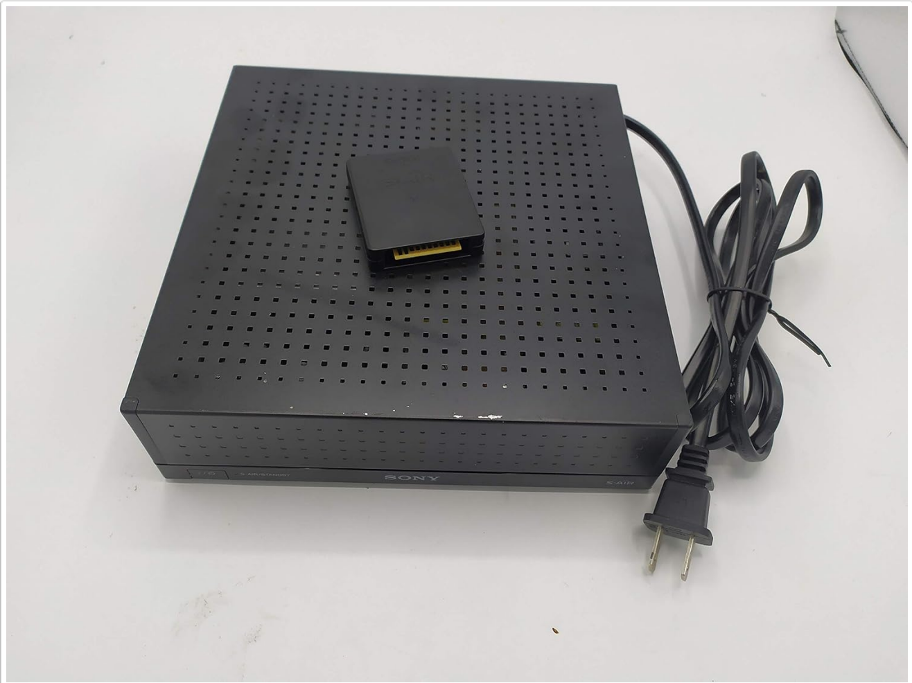
Figure 2.1: Front view of the Sony TA-SA200WR Wireless S-Air Surround Amplifier, showing the main unit and the S-Air wireless transceiver module.
