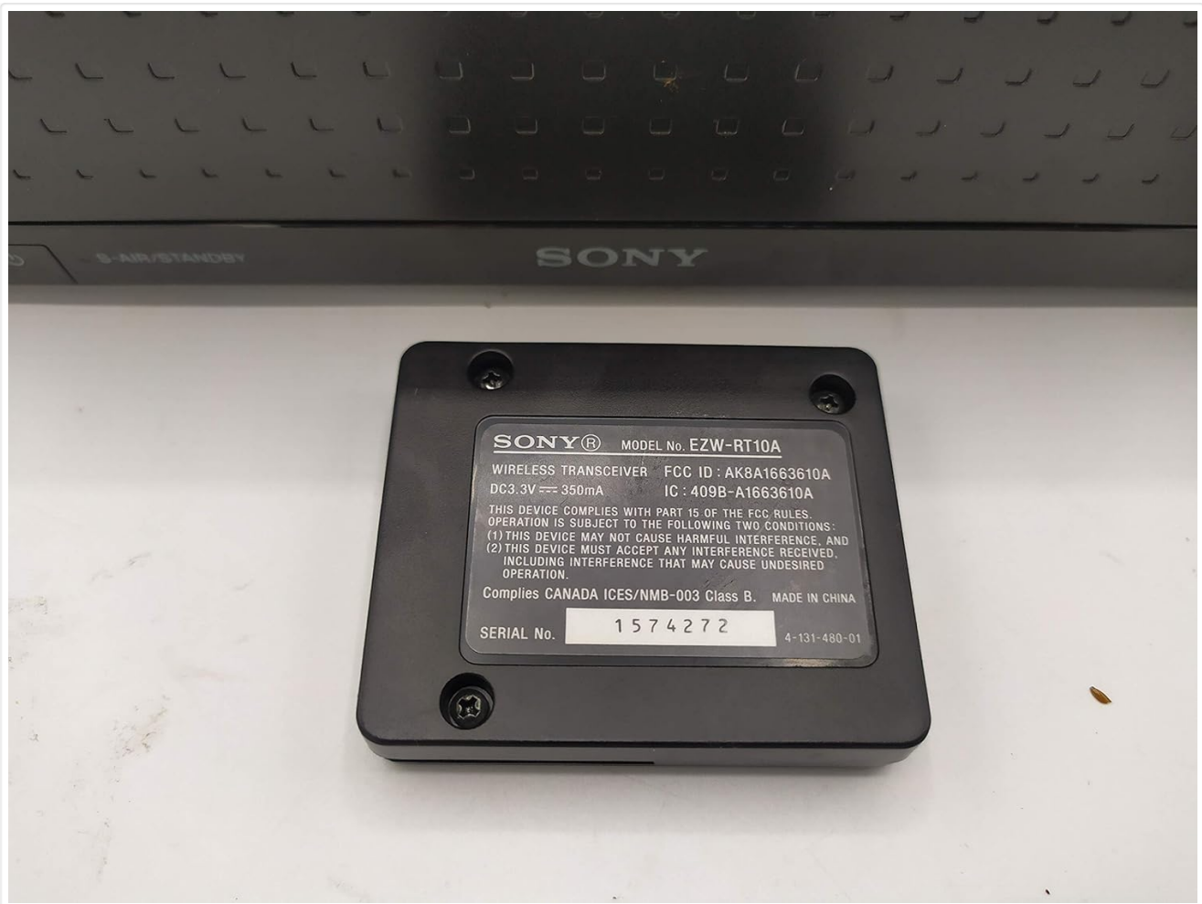
Figure 2.3: The EZW-RT10A wireless transceiver module, which plugs into the amplifier to enable S-Air communication.
