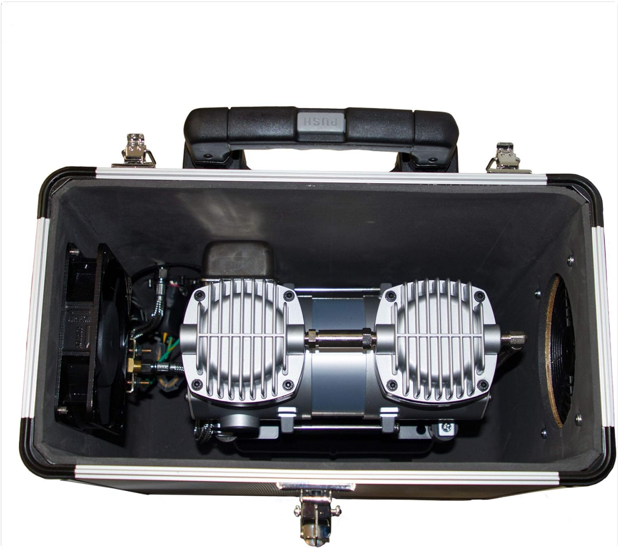
Figure 3.2: Internal view of the Sparmax MB-620 compressor unit and fan within the case.
