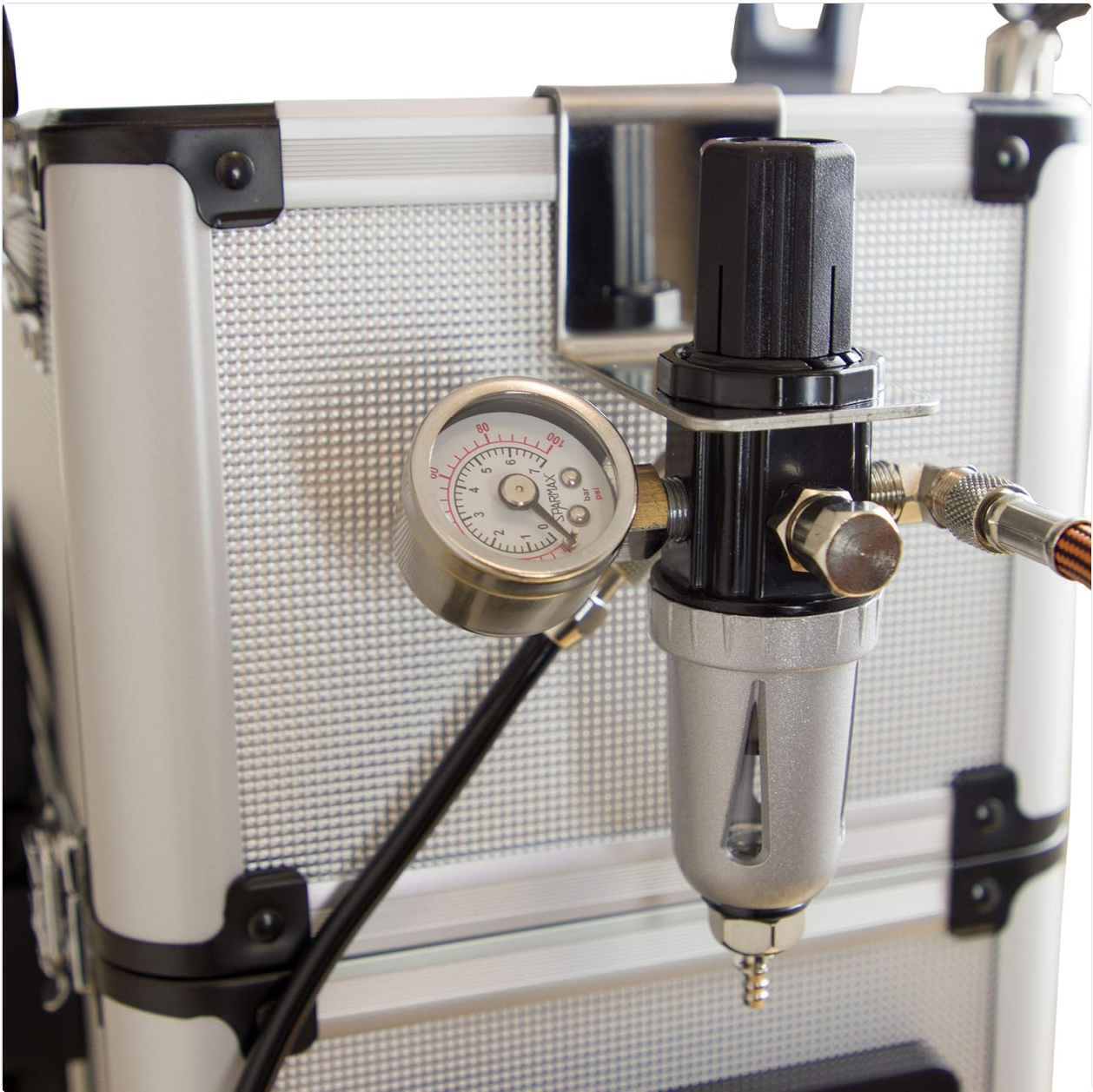
Figure 3.3: Close-up of the pressure regulator, water trap, and pressure gauge.
