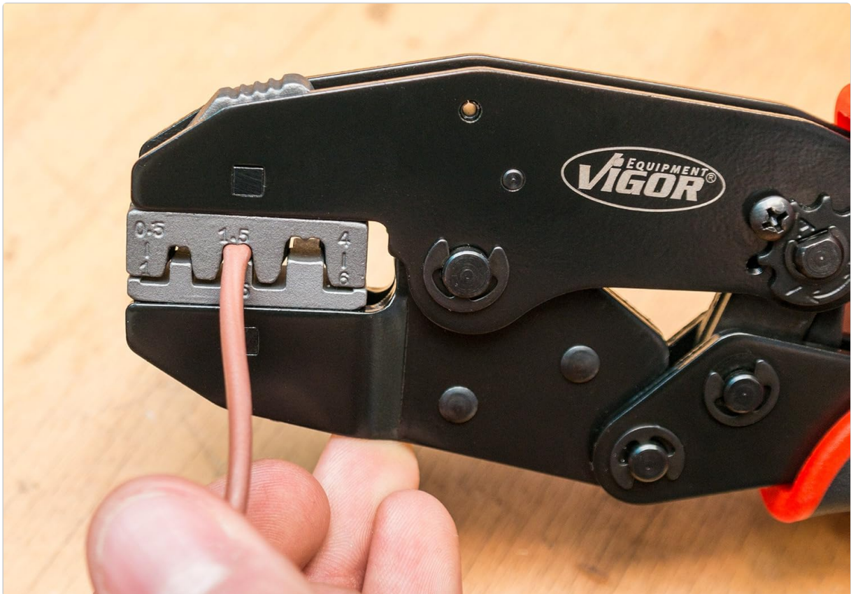
Image: A close-up of the Vigor V2499 crimping pliers showing a brown wire positioned within a crimping cavity, with wire gauge markings (0.5, 1.5, 4) visible on the insert.
