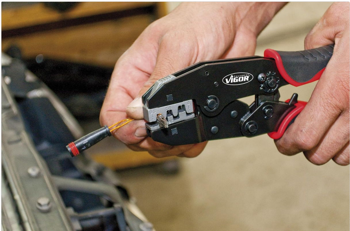
Image: A hand holding the Vigor V2499 crimping pliers, preparing to crimp a wire with insulation stripped, showing the wire being inserted into a terminal.
