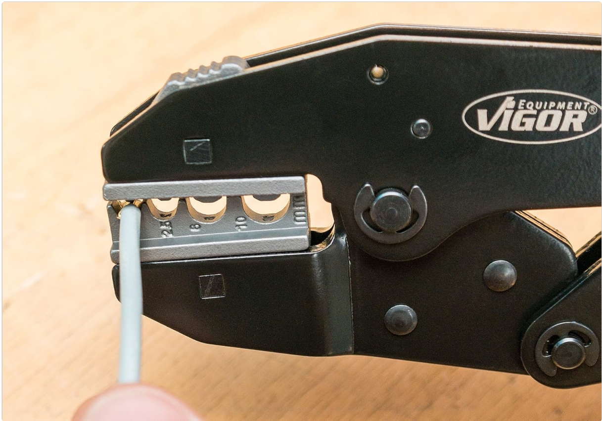
Image: A close-up of the Vigor V2499 crimping pliers showing a wire being inserted into a crimping cavity, with the numerical markings for wire gauges visible on the insert.
