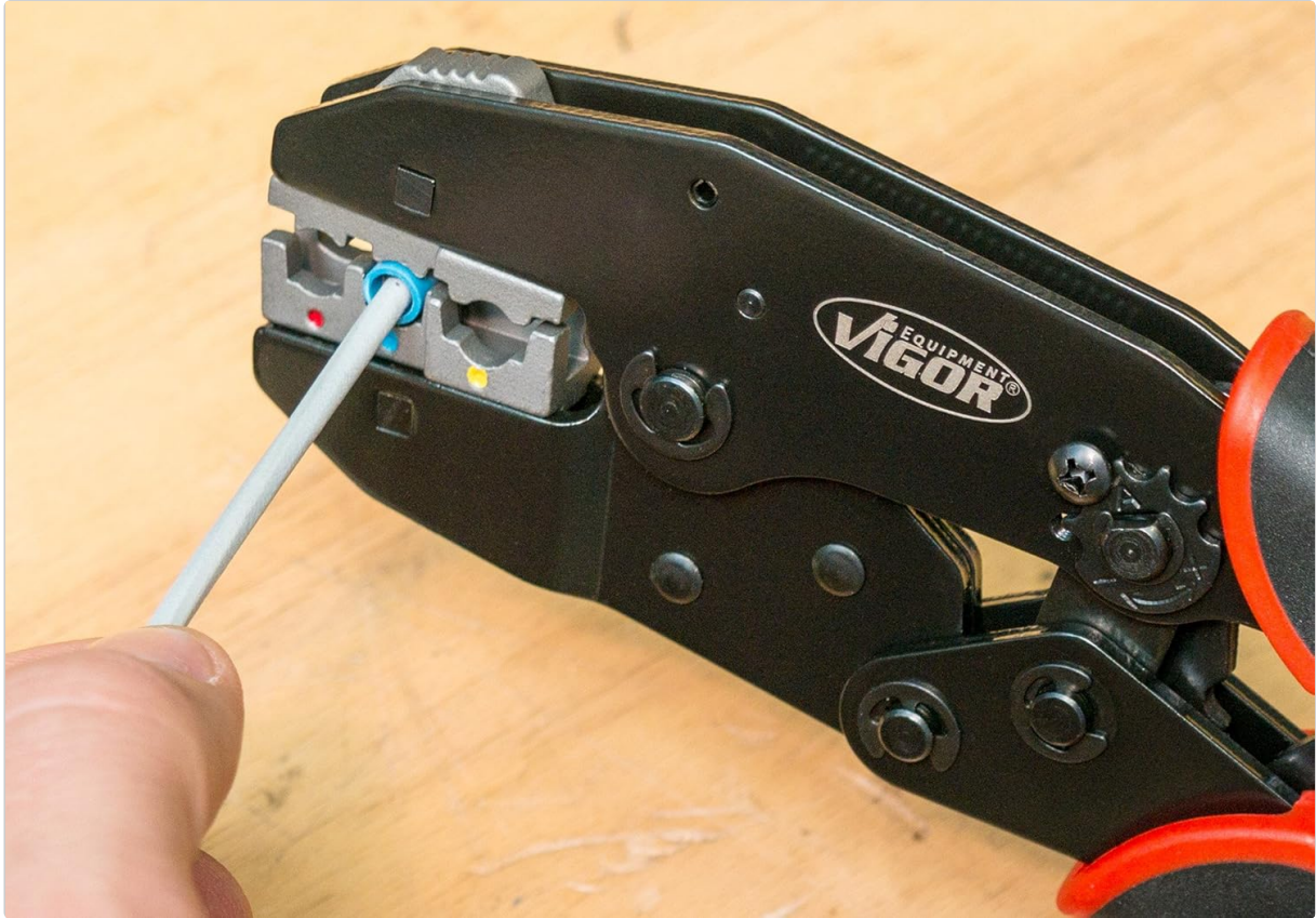
Image: A close-up of the Vigor V2499 crimping pliers showing a wire being placed into a specific color-coded crimping cavity on an installed insert.
