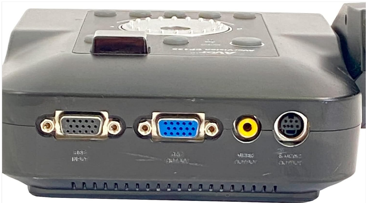
Figure 4.4: Rear Connectivity Ports. This image shows the various input and output ports on the rear of the base unit, including VGA input (RGB INPUT), VGA output (RGB OUTPUT), Composite Video output (VIDEO OUTPUT), and S-Video output (S-VIDEO OUTPUT).
