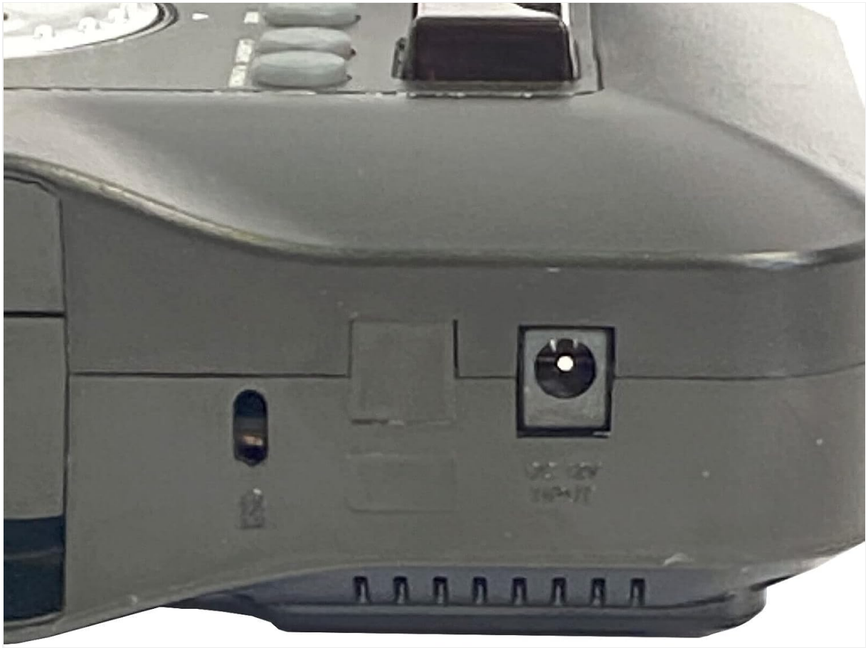
Figure 4.6: DC 12V Power Input. A close-up of the DC 12V power input port located on the side of the base unit, where the power adapter connects.
