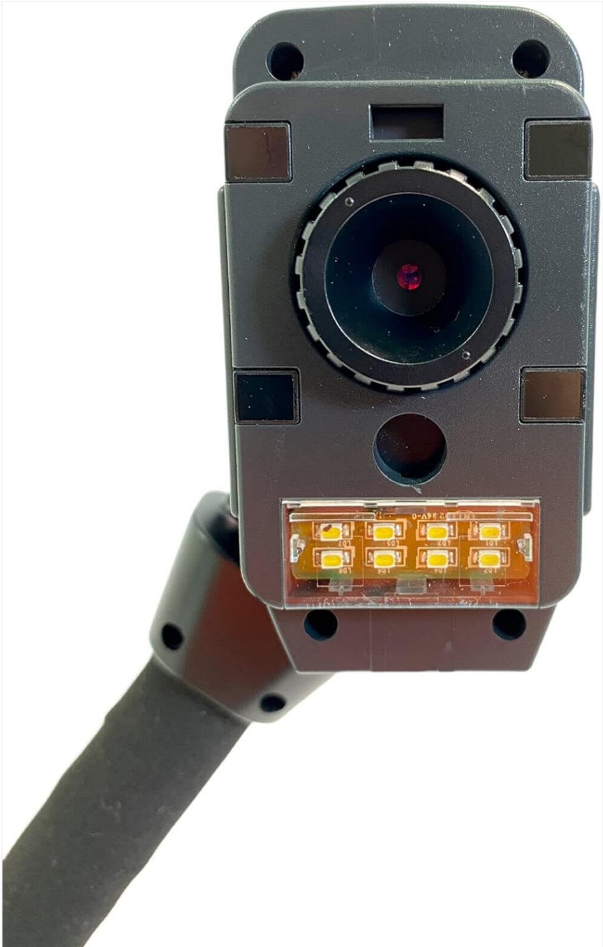
Figure 4.3: Camera Head with Integrated LED Lighting. A close-up of the camera lens and the built-in LED lights, which provide illumination for clear image capture, especially in low-light conditions.
