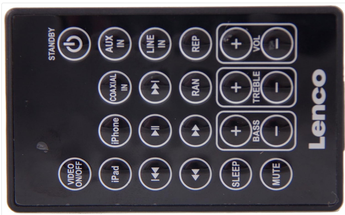
Figure 5: The remote control for the Lenco iPD-1003, featuring buttons for standby, AUX in, line in, coaxial in, video on/off, iPod/iPhone/iPad control, volume, bass, treble, and mute functions.
