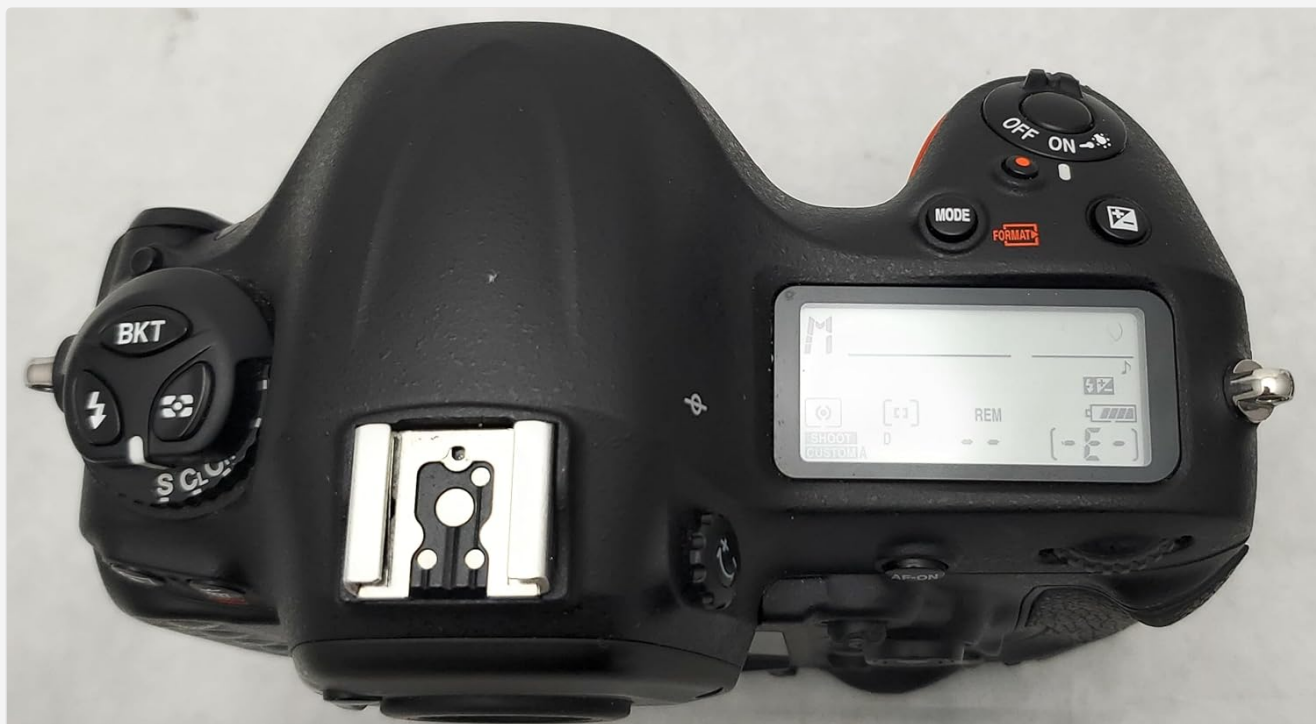
Figure 3.1.1: Top view of the Nikon D4 camera, displaying the top LCD panel and various control buttons for settings like mode, exposure compensation, and metering.
