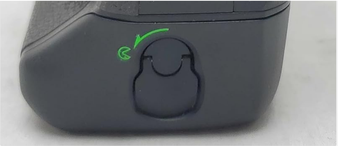
Figure 3.2.1: Left side of the Nikon D4 camera, revealing the port covers for USB, HDMI, microphone input, and headphone output, essential for video recording and connectivity.
