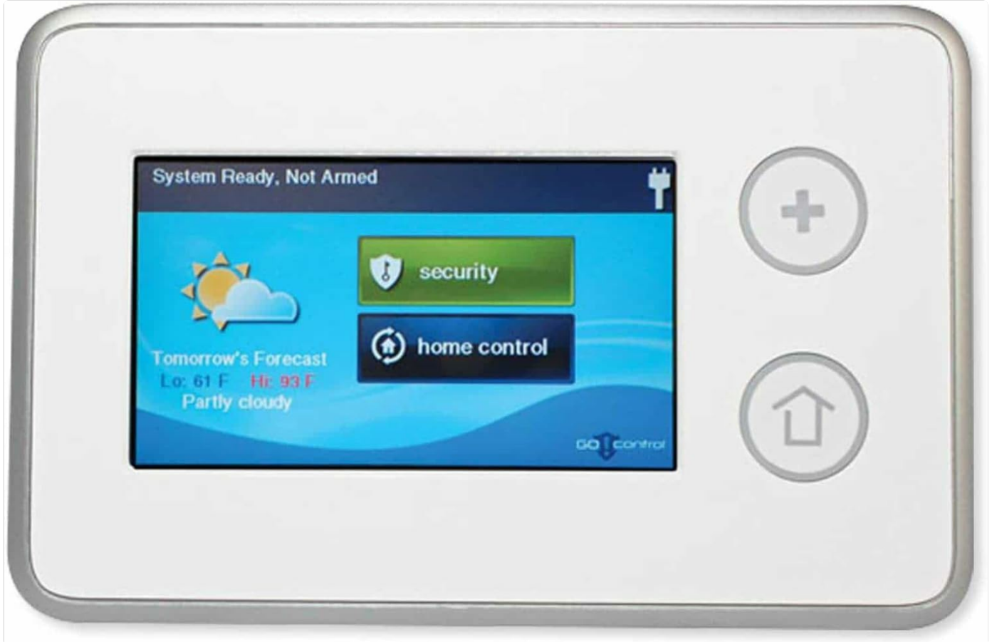
Figure 2: The main screen of the TS1 keypad, showing system status and primary navigation options.
