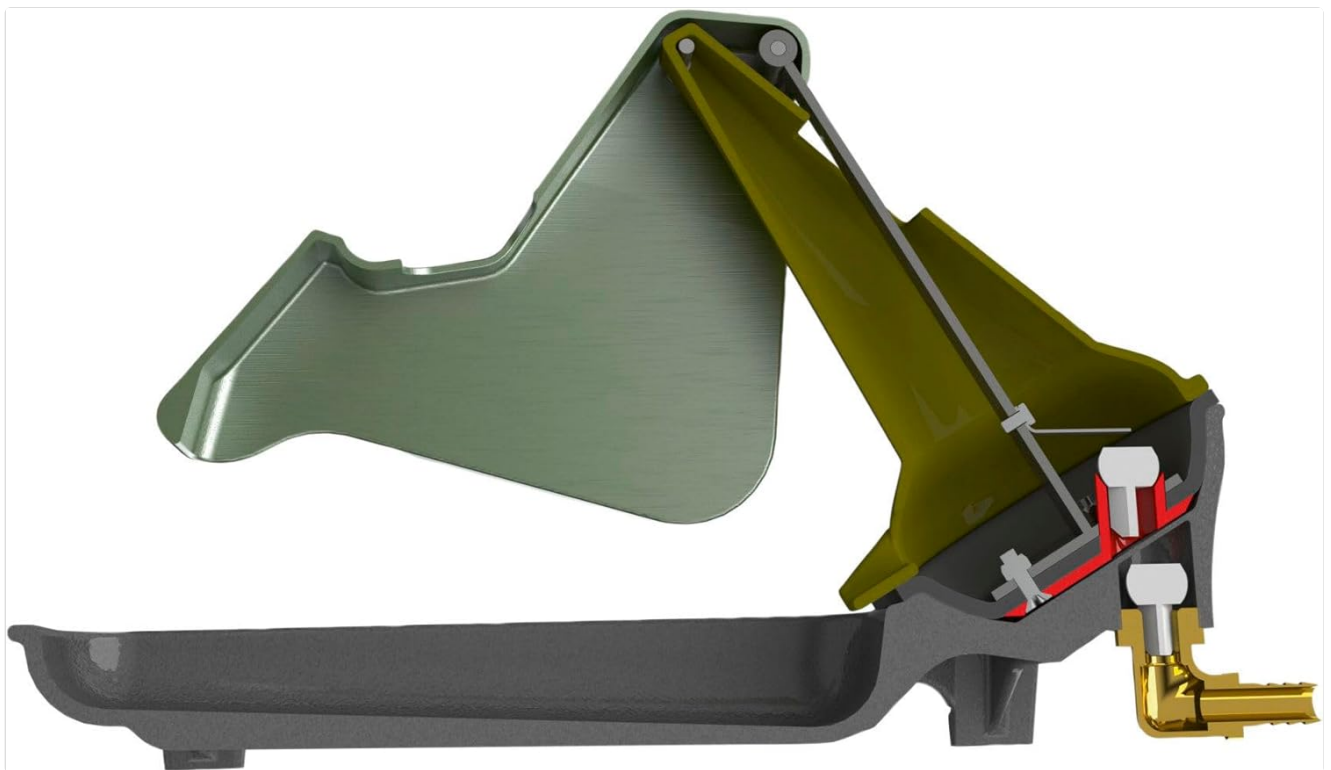
Figure 2: Internal mechanism of the Kerbl P100 Willow Pump, highlighting the lever, piston, and valve system responsible for water suction and delivery.
