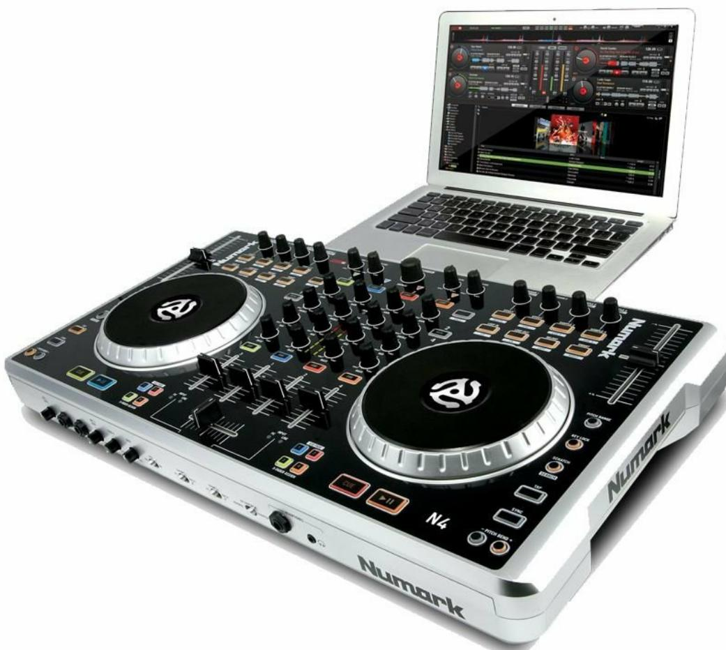
A comprehensive top-down view of the Numark N4 controller, showcasing its dual jog wheels, 4-channel mixer section with faders and EQ knobs, performance pads, and navigation controls for seamless DJing.
