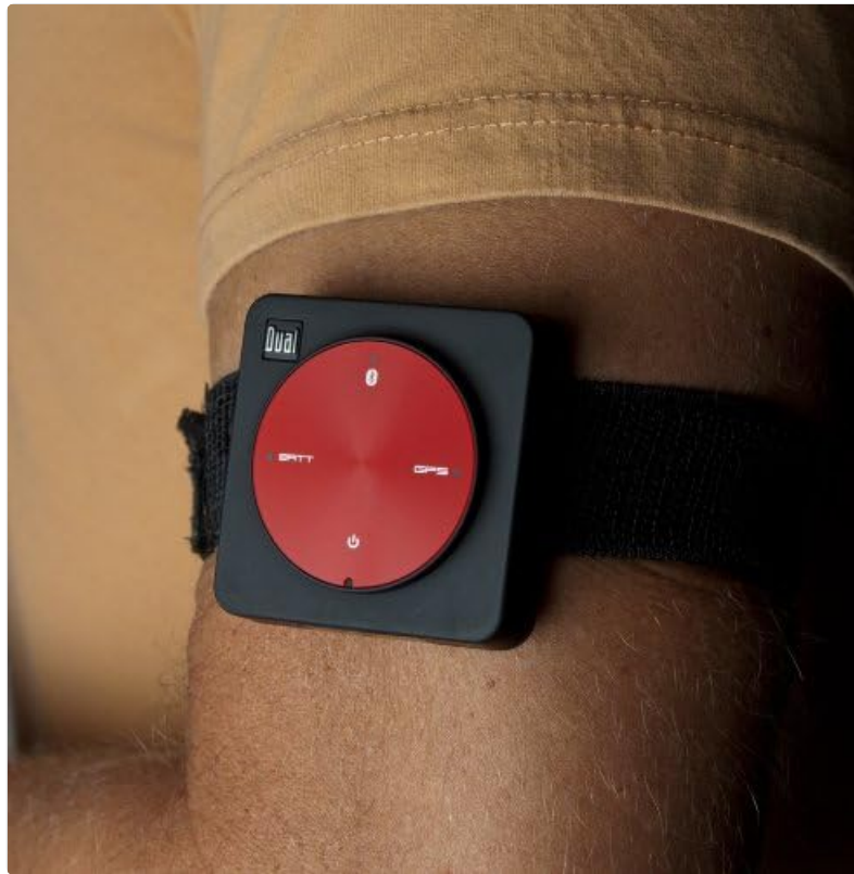
Figure 5: The XGPS150A secured to a user's arm using the adjustable strap, suitable for outdoor activities like hiking or running.
