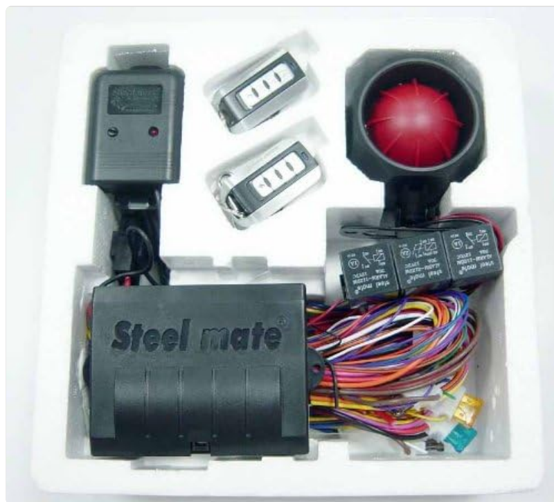
Figure 3.2: All components of the Steelmate 858 system laid out for inspection.
