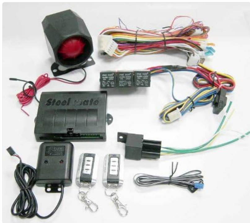
Figure 3.3: Key components including the main unit, siren, starter relay harness, and shock sensor.
