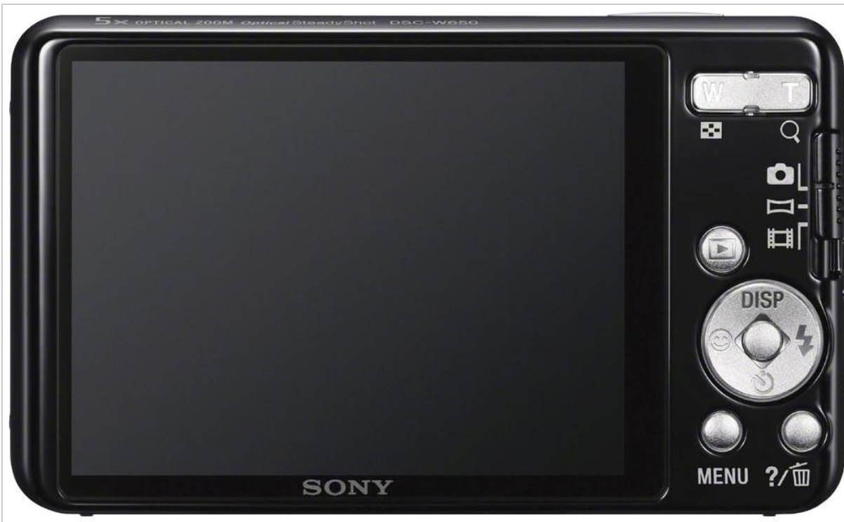
Figure 2: Rear view of the Sony Cyber-shot DSC-W650 digital camera. This image shows the camera's back panel, featuring the large 3.0-inch LCD screen, the zoom lever (W/T), the playback button, the DISP button, the 5-way control button, and the MENU button. The 'SONY' logo is also present at the bottom.
