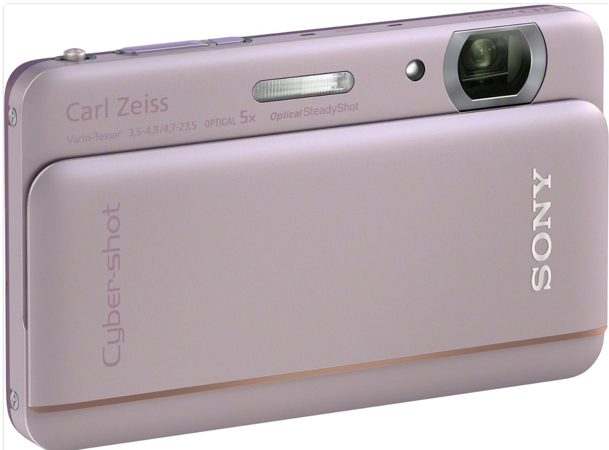
Figure 2: Sony Cyber-shot DSC-TX66 camera with the front cover slid down, revealing the lens and flash.
