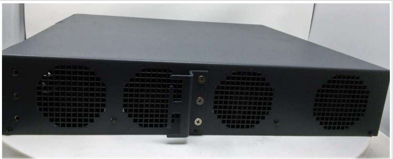
Figure 8.4: Side view of the Avaya G700 Media Gateway, showing the ventilation grilles. These grilles are crucial for proper airflow and cooling of the internal components.
