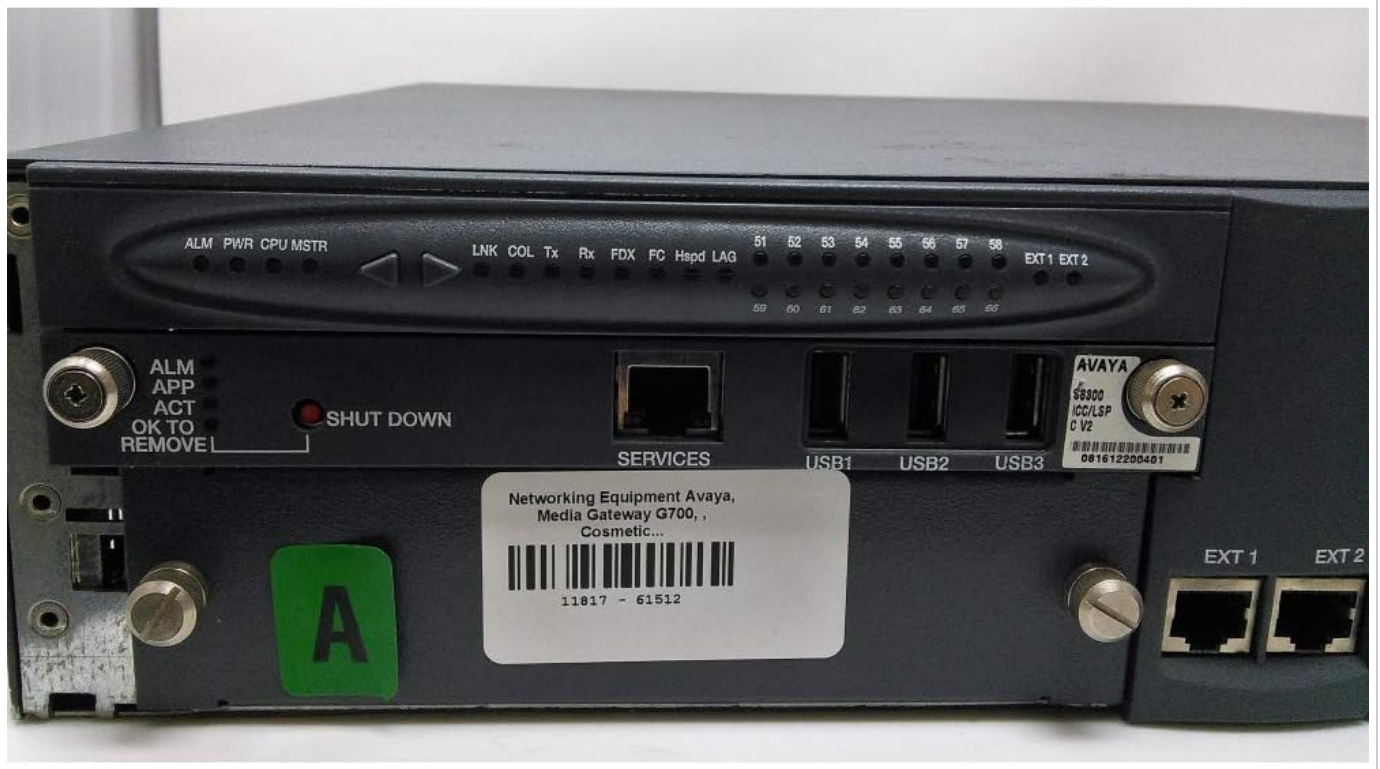
Figure 8.3: Close-up view of the Avaya G700 Media Gateway front panel. This detailed image highlights the status LEDs (ALM, PWR, CPU, MSTR, LNK, COL, Tx, Rx, FDX, PC, Hspd, LAG), USB ports, SERVICES port, and module slots.
