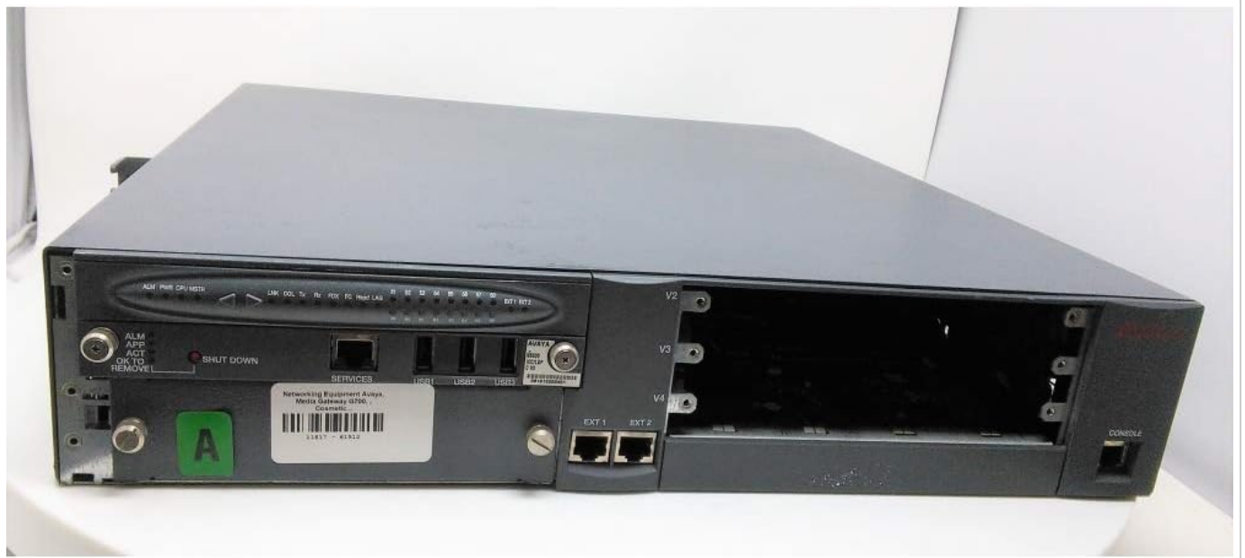
Figure 8.1: Front and top view of the Avaya G700 Media Gateway. This image displays the overall chassis, including the front panel with status indicators and module slots, and the top casing.
