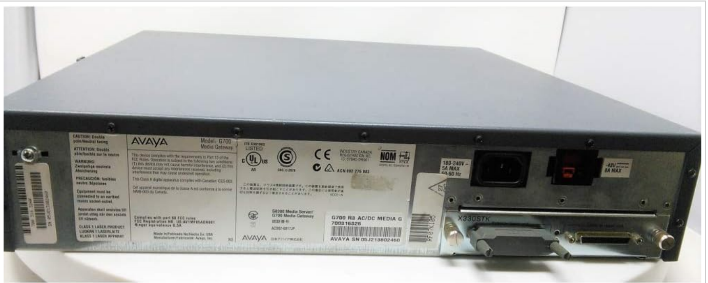
Figure 8.2: Rear view of the Avaya G700 Media Gateway. This view shows the power input, various regulatory labels, and additional connectivity ports on the back panel.
