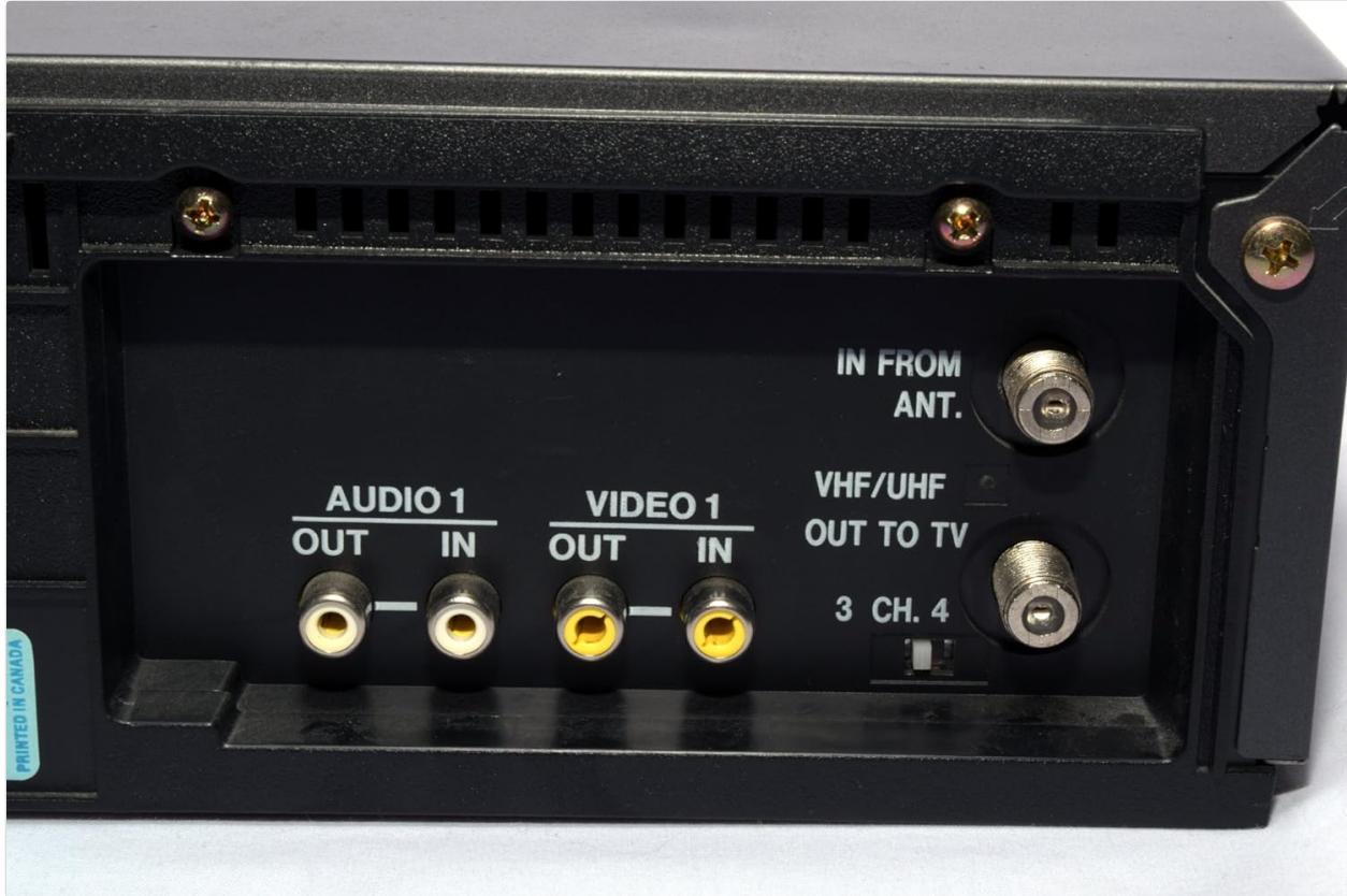
This image displays the rear panel of the VCR, highlighting the 'AUDIO 1 OUT/IN' (white and red RCA), 'VIDEO 1 OUT/IN' (yellow RCA), 'IN FROM ANT.' (RF coaxial), and 'VHF/UHF OUT TO TV' (RF coaxial with CH. 3/4 switch) ports. These are crucial for connecting the VCR to your television and antenna or cable source.
