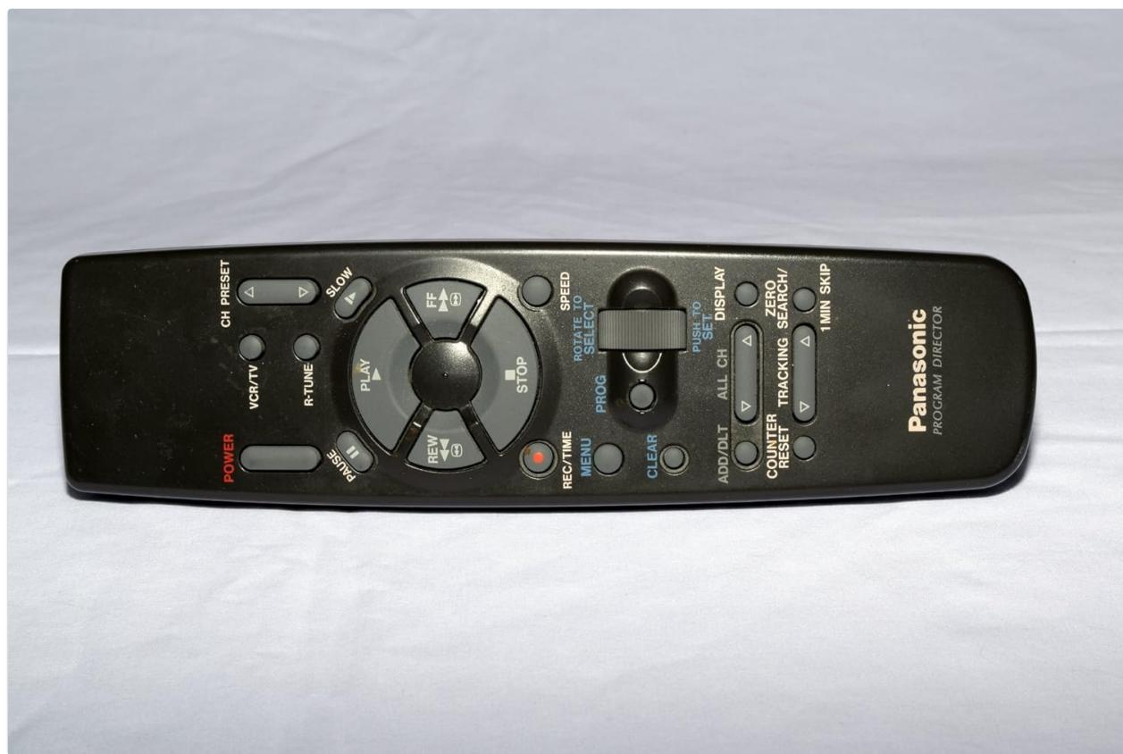
The remote control features buttons for power, channel selection (CH PRESET, CH UP/DOWN), VCR/TV mode, playback controls (PLAY, STOP, REW, FF, PAUSE), recording (REC/TIME MENU), tracking, and display functions. This remote is essential for convenient operation of the VCR.
