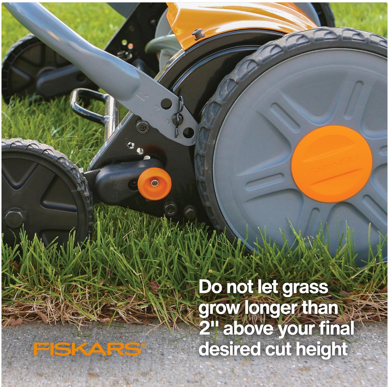
Figure 4: Guidance on maintaining appropriate grass height for effective cutting.
