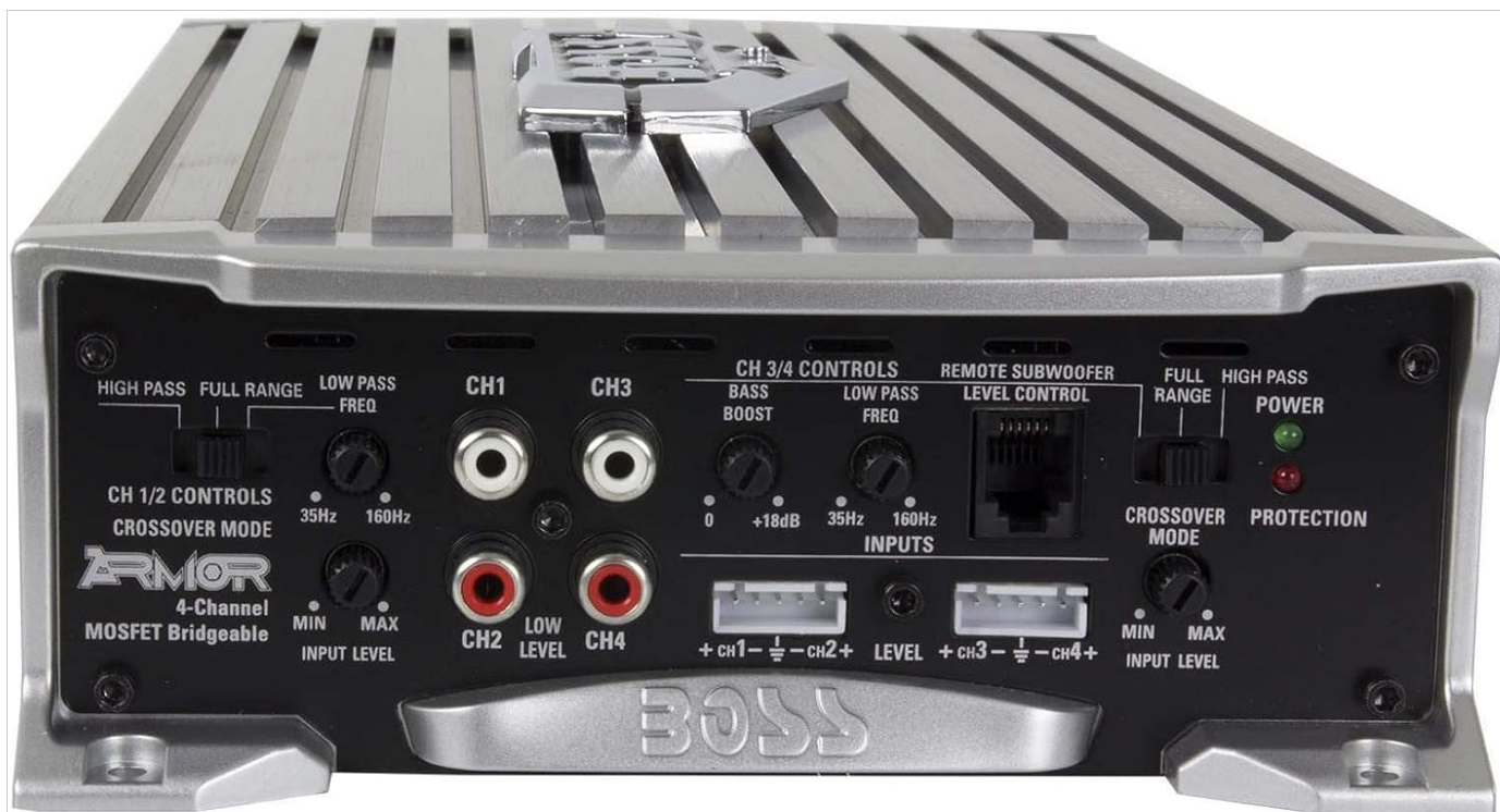
Image: Front control panel of the BOSS AR1600.4 amplifier, displaying the CH 1/2 and CH 3/4 Crossover Mode switches, High Pass/Full Range/Low Pass frequency controls, Bass Boost, Input Level adjustments, and the Remote Subwoofer Level Control port.
