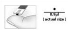
Figure 3: This diagram shows a finger with a blood drop being touched to the edge of a test strip, demonstrating the proper blood application technique. The required blood volume of 0.9 \mu\text{L} is also indicated.
