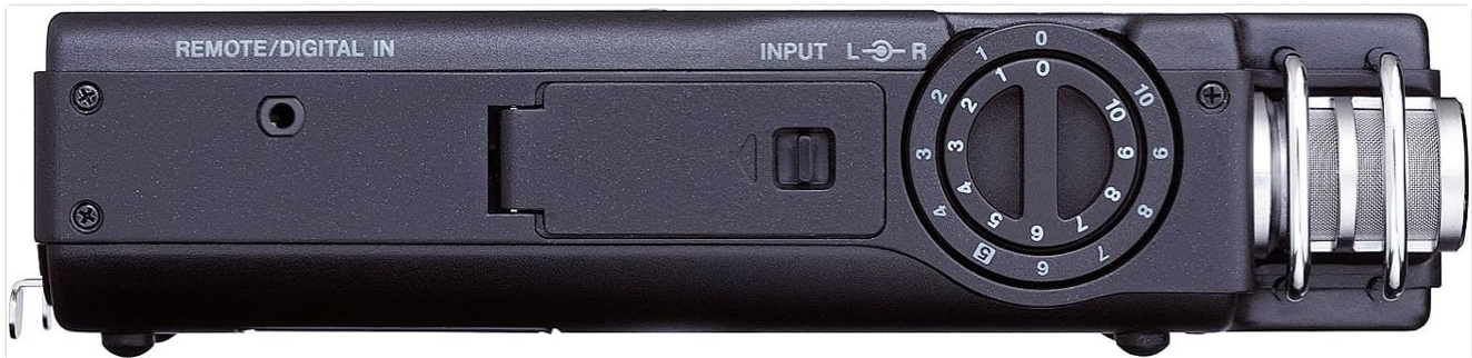
Figure 6: Top view of the DR-100MKII, illustrating the large rotary input volume dials for precise left and right channel gain adjustment.
