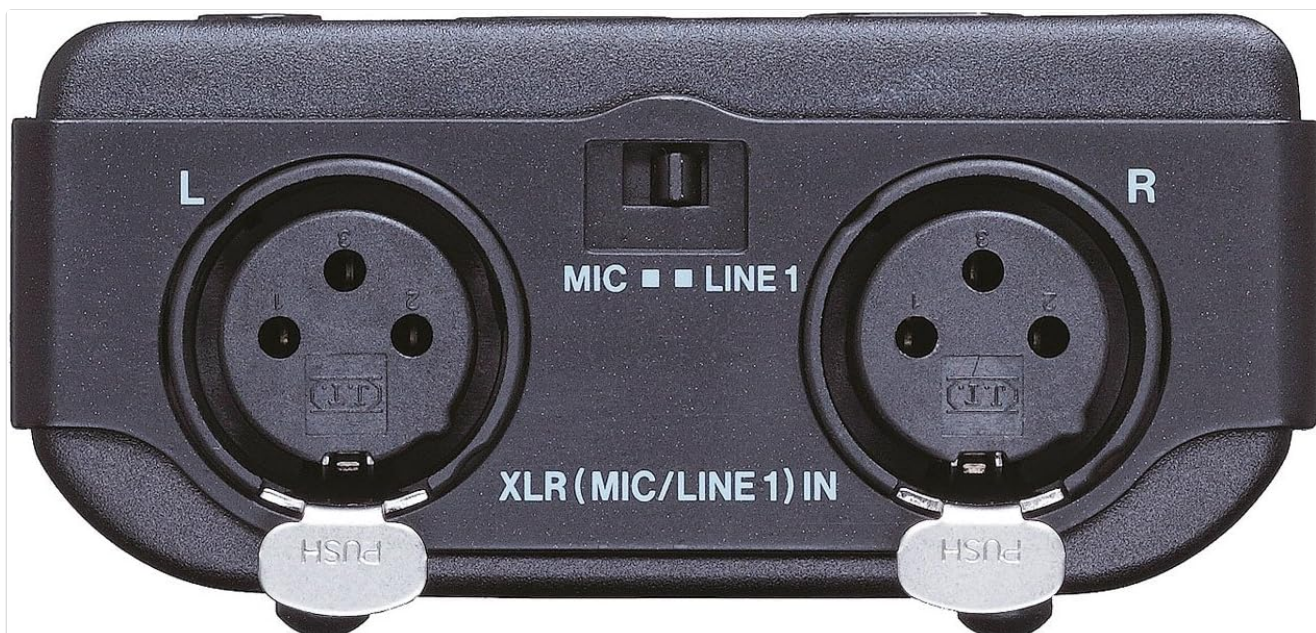
Figure 3: Close-up view of the DR-100MKII's bottom, showing the locking XLR (MIC/LINE 1) inputs for professional audio connections.
