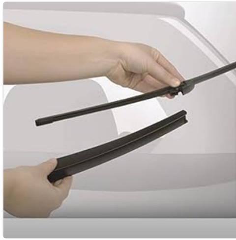
Figure 2: Illustration of detaching an old wiper blade from the arm.
