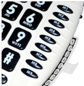
Figure 3: Detail of the memory buttons (M1-M9) and the integrated memory index card.
