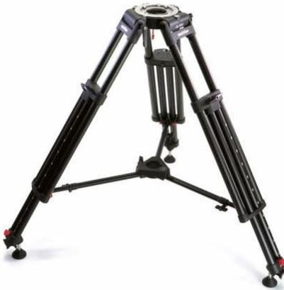
Figure 1: The Sachtler OB 2000 tripod in an extended position, showcasing its robust aluminum construction, two-section legs, and flat base for mounting a camera head. The integrated spreader and rotating rubber feet are also visible.
