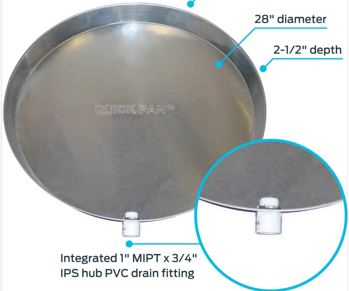
Figure 2: Key specifications of the Holdrite QuickPan.
