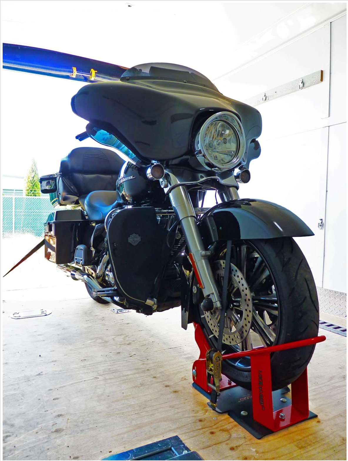
Figure 7: Side view illustrating the motorcycle's position in the chock.
