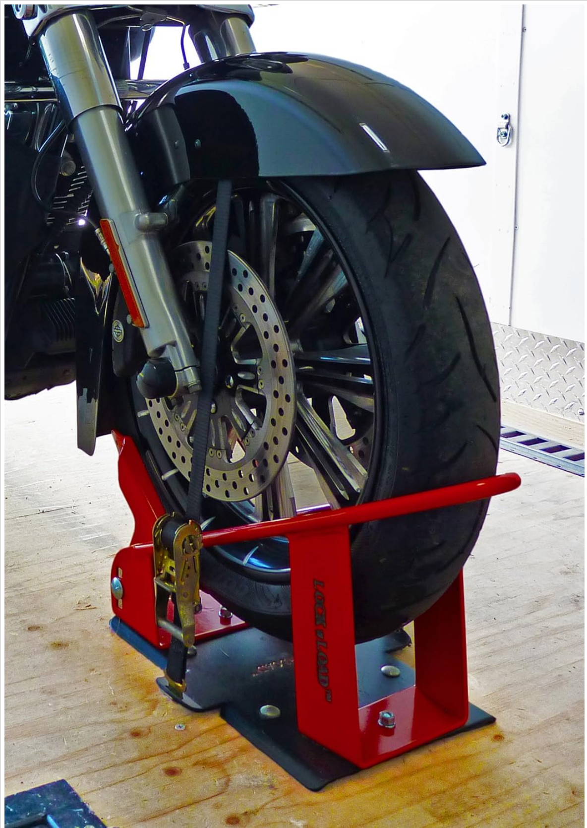
Figure 8: Close-up of the front wheel secured by the chock and tie-down strap.
