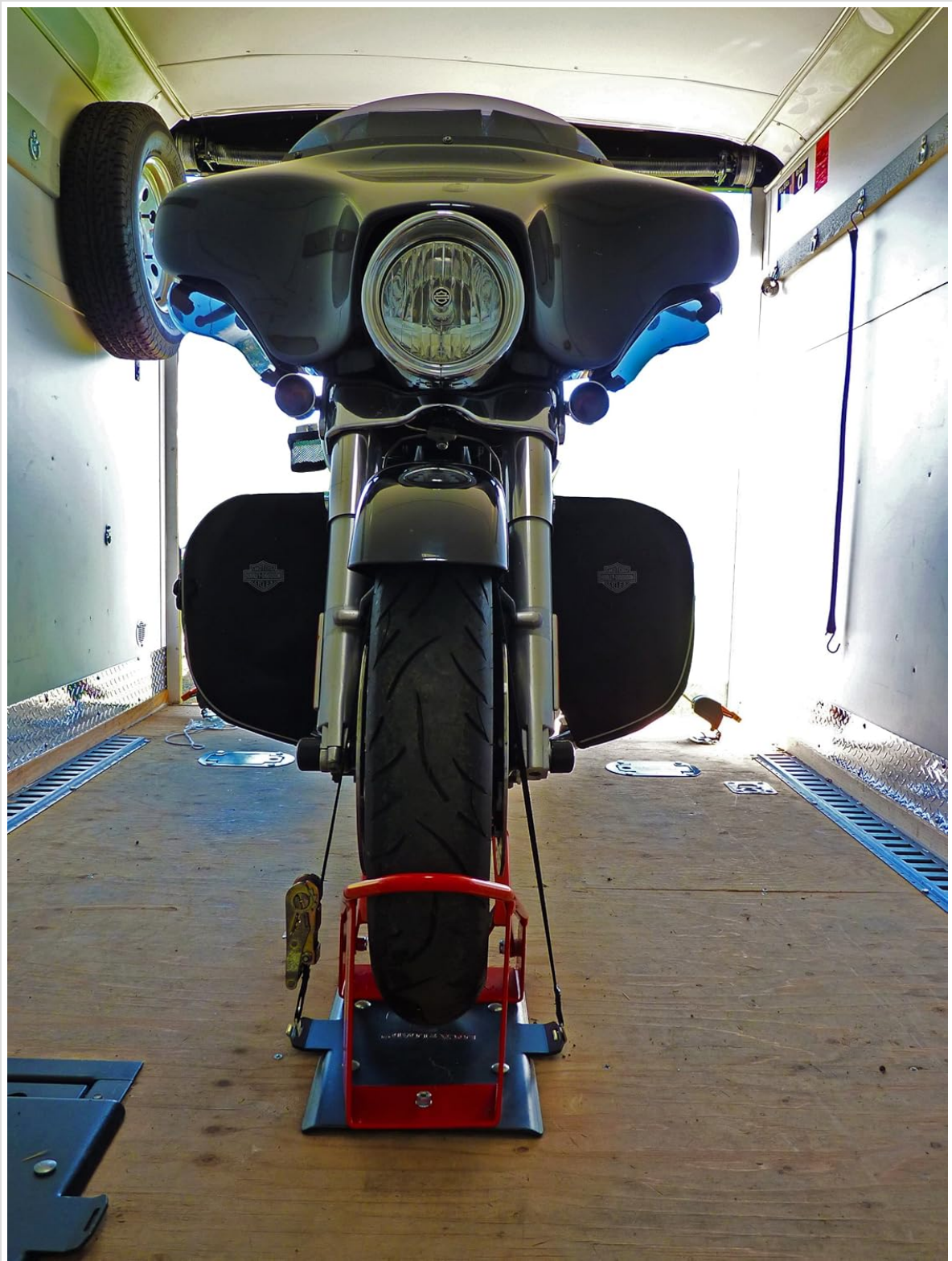
Figure 6: Front view of a motorcycle securely loaded in the chock.
