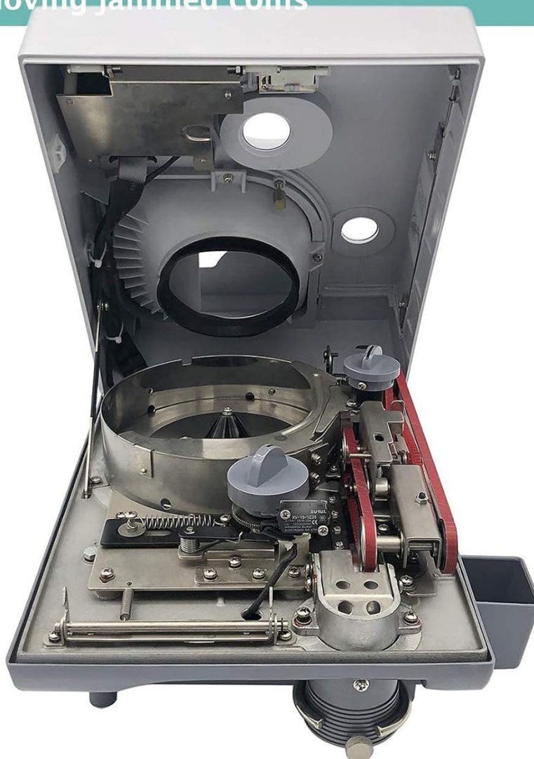
Figure 7.1: The Coin-Mate CS-2000 with its front panel open for easy access to internal components for cleaning.
