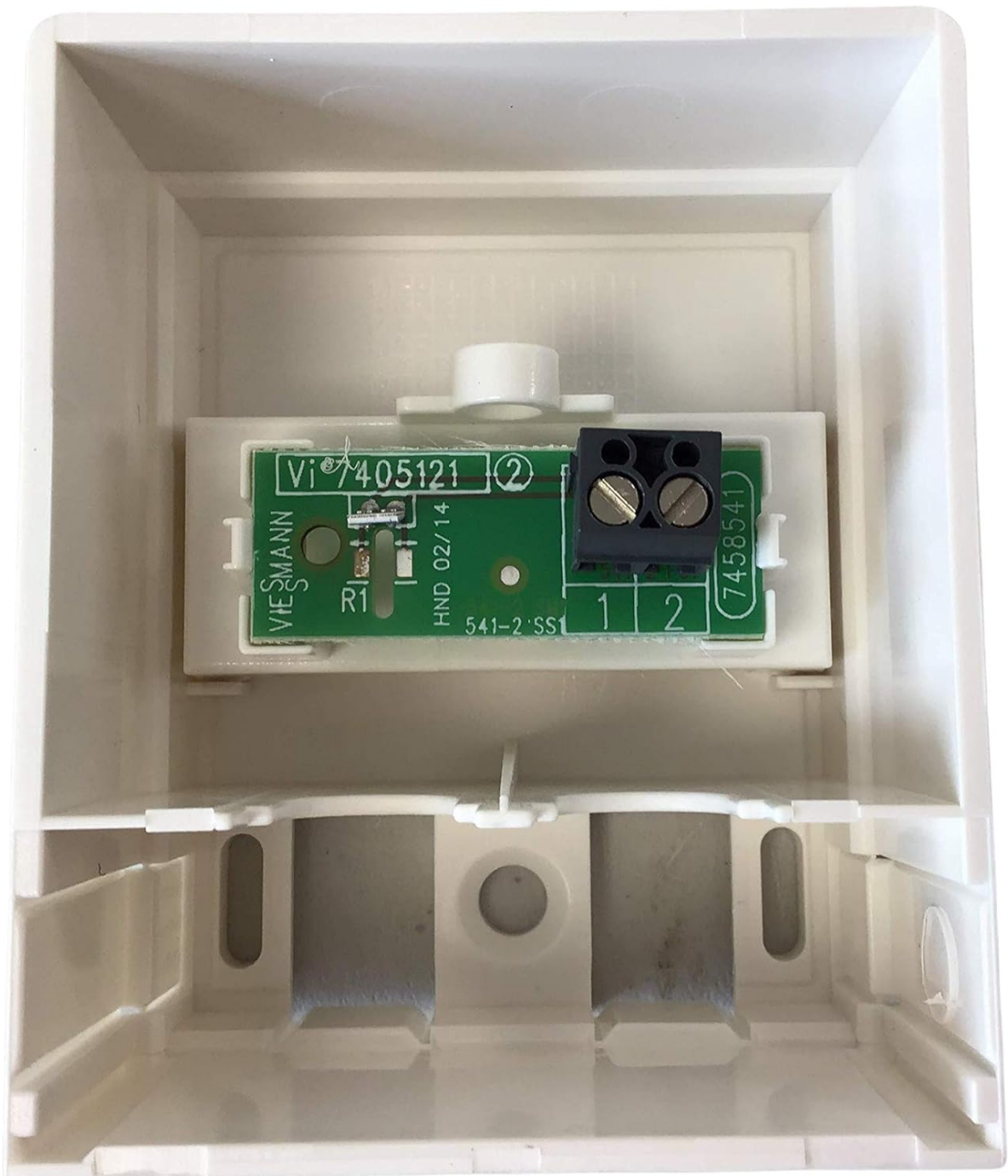
Image: Close-up view of the Viessmann 7820148 Outdoor Sensor #1's internal circuit board. The green board has 'VIESSMANN' printed on it, along with 'HND 02/14' and terminals labeled '1' and '2' for wiring connections.
