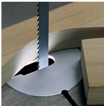
Figure 2: A band saw blade properly installed and positioned in the saw's guides.
