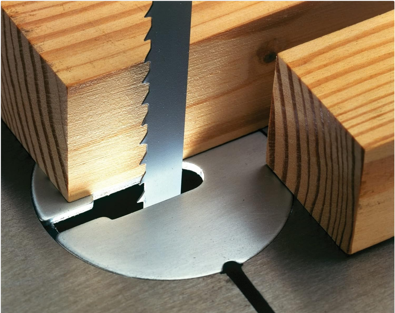
Figure 3: The BOSCH BS80-6W blade actively cutting a wooden workpiece on a band saw.
