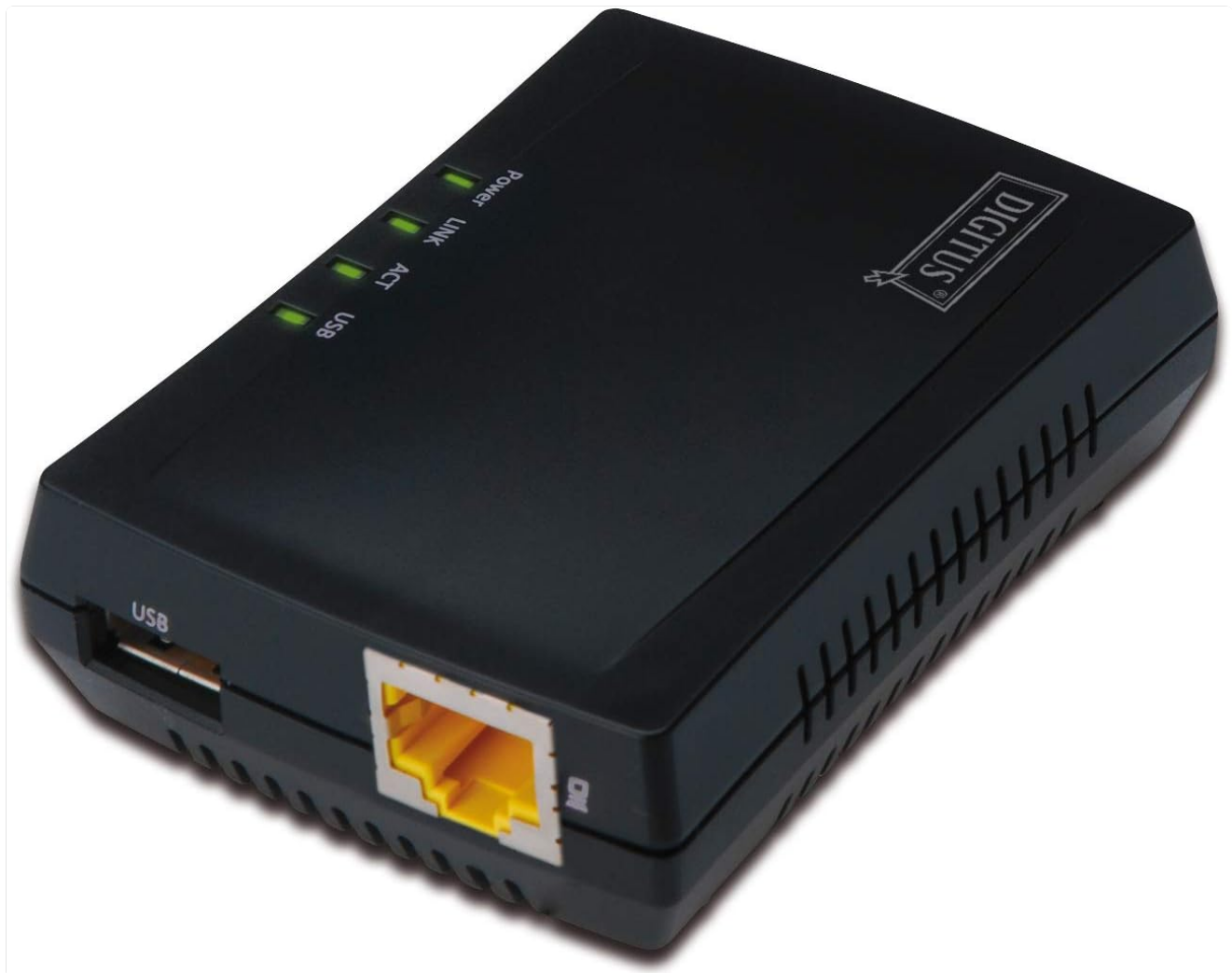
Figure 4.1: Top-down view of the Digitus Multifunction Network Server, showing LED indicators for Power, Link, ACT, and USB.
